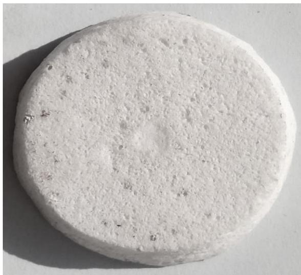
Fig. 6. Sample of heat insulating coating containing 70 wt % of foamed binder and 30 wt. % of filler.
