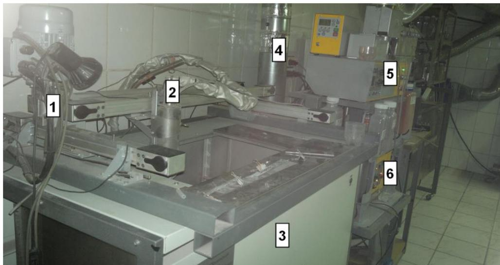
**Fig. 3. Assembly for application of heat insulating coatings on the basis of microspheres and anisotropic nanostructures: 1 - 3-axial positioning system; 2 – meter; 3 – dust proof chamber; 4 – air removal and cleaning duct; 5 – control unit of positioning system; 6 – unit for application of multilayer coatings.**
