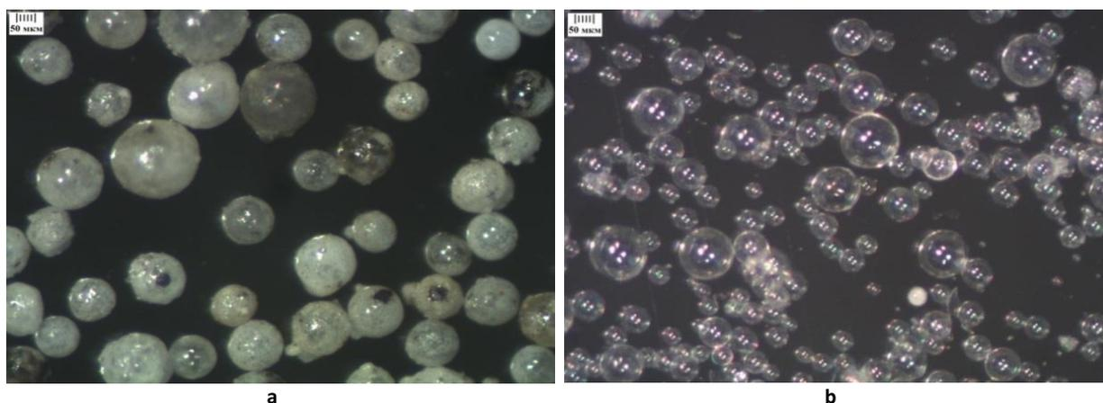
Fig. 1. Appearance of microspheres: a -- aluminosilicate; b -- sodium borosilicate.
