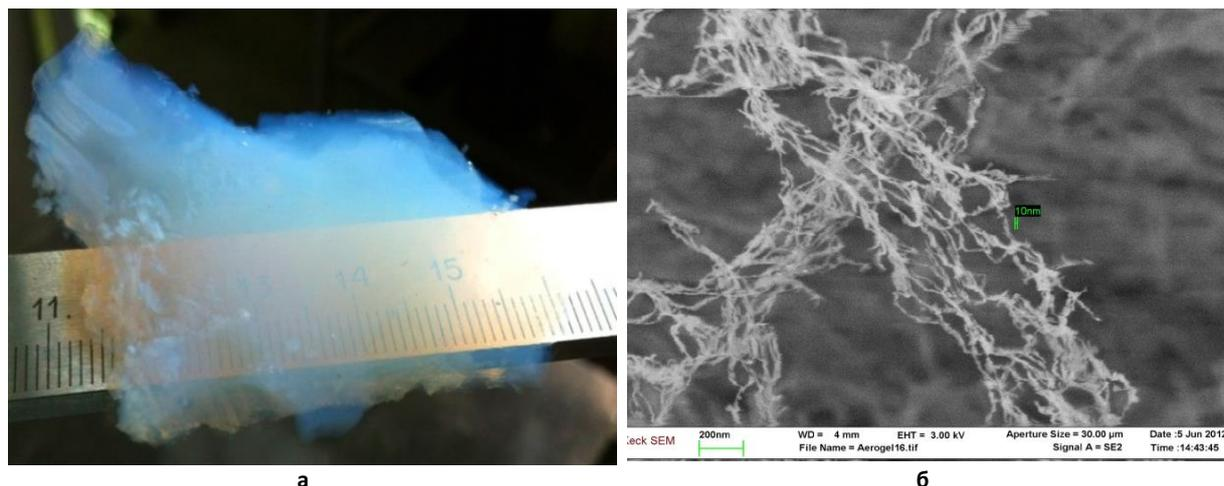
**Fig. 2. Appearance and structure of AIOOH aerogel: a -- appearance of AIOOH aerogel sample with the size of 40×25×8 mm; b -- microstructure of AIOOH aerogel, 4000× magnification.**
