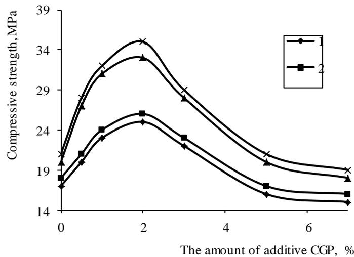
**Figure 5: Compressive strength of sulfuric-silica compositions, modified by CGP obtained by technology: vibro-packing (1, 2) and compression (3, 4), with different contents of modifying additive CGP and time of synthesis: 1, 3-30 minutes; 2, 4-60**
