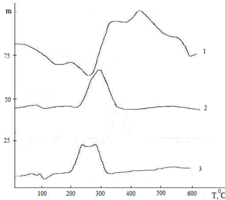
Figure 11: The curves of differential thermal analysis of calcium glycerophosphate (1), sulfur (2) and compositions based on them (3)
