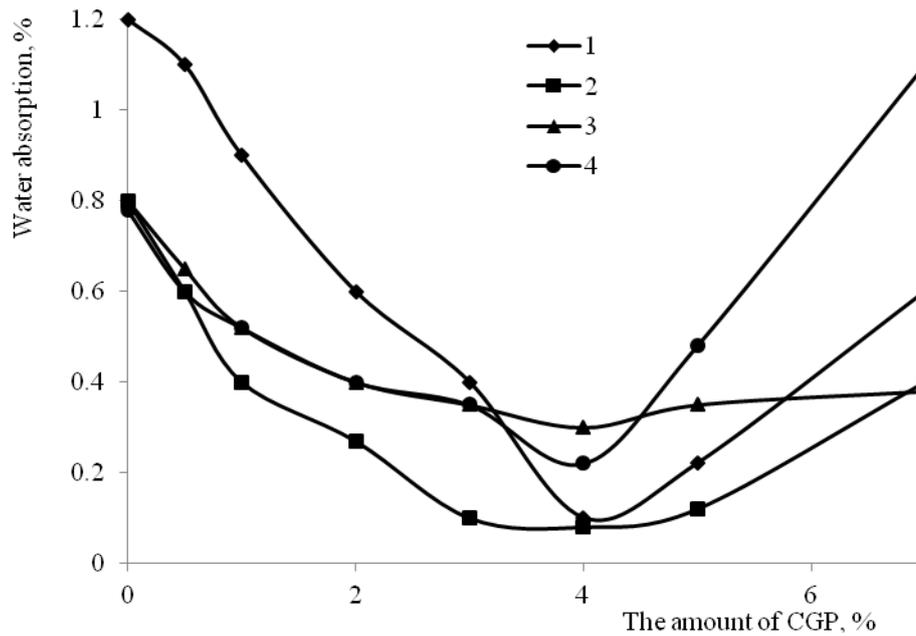
Figure 7: Dependence of water absorption of sulfuric-ash-and-slag samples with modifying additive calcium glycerophosphate from amount of additive and time samples synthesis: 1– 10 min, 2 – 30 min, 3 – 1 hour, 4 – 2 hours
