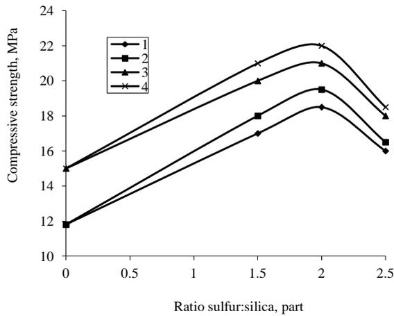
Figure 1: Compressive strength of binary sulfur silica compositions, produced by vibro packing (1, 2) and compression (3, 4) at various ratios of components and time of synthesis samples: 1, 3-30 min; 2, 4-60 min.
