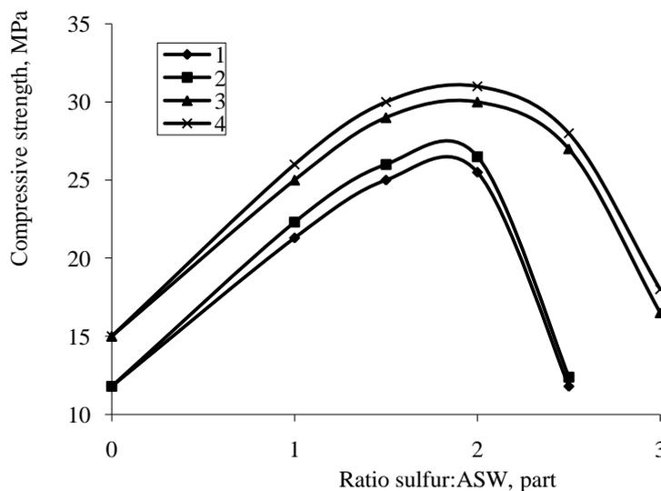
Figure 2: Compressive strength of binary sulfur ash-and-slag waste compositions, produced by vibro packing (1, 2) and compression (3, 4) at various ratios of components and time of samples synthesis: 1, 3-30 min; 2, 4-60 min.
