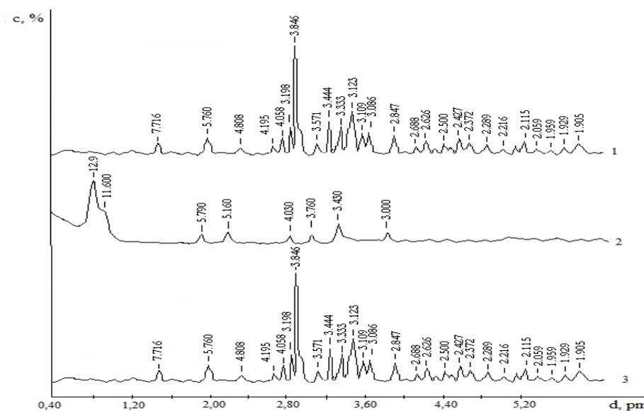
Figure 9: Roentgenogram of sulfur samples (1), calcium glycerophosphate (2) and polysulfide material with the addition of calcium glycerophosphate (3)
