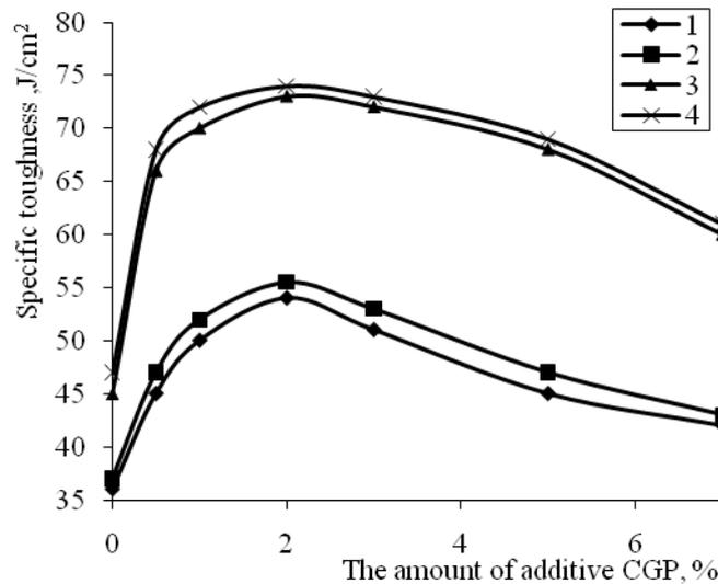
Figure 8: The dependence of the specific toughness of sulfuric-silica (1, 2) and sulfuric ash-and-slag (3, 4) compositions, modifying by CGP at different contents of modifying additive CGP and synthesis time: 1,3 – 30 min; 2,4 – 60 min.
