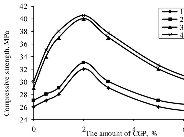
**Figure 6: Compressive strength of sulfuric-ash-and-slag compositions, modified by CGP obtained by technology: vibro-packing (1, 2) and compression (3, 4), with different contents of modifying additive CGP and time of synthesis: 1, 3-30 minutes; 2, 4-60**
