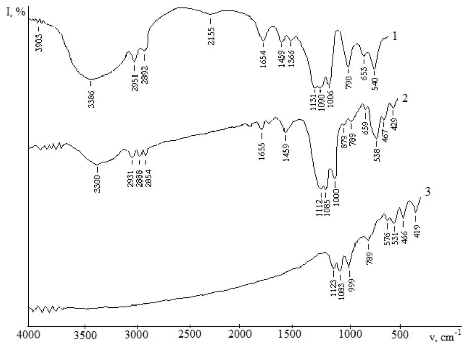
Figure 12: IR spectra of the samples of calcium glycerophosphate (1), and polysulfide compounds with addition of calcium glycerophosphate of a small synthesis time (2) and the long lasting time of synthesis (3)
