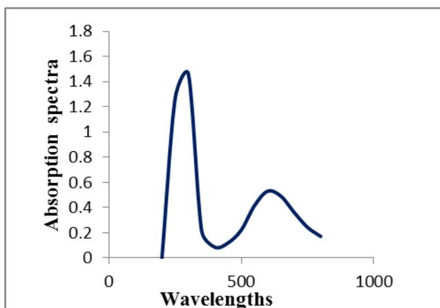
Figure 1: UV-Vis absorption spectra of Copper NPs at various wavelengths
