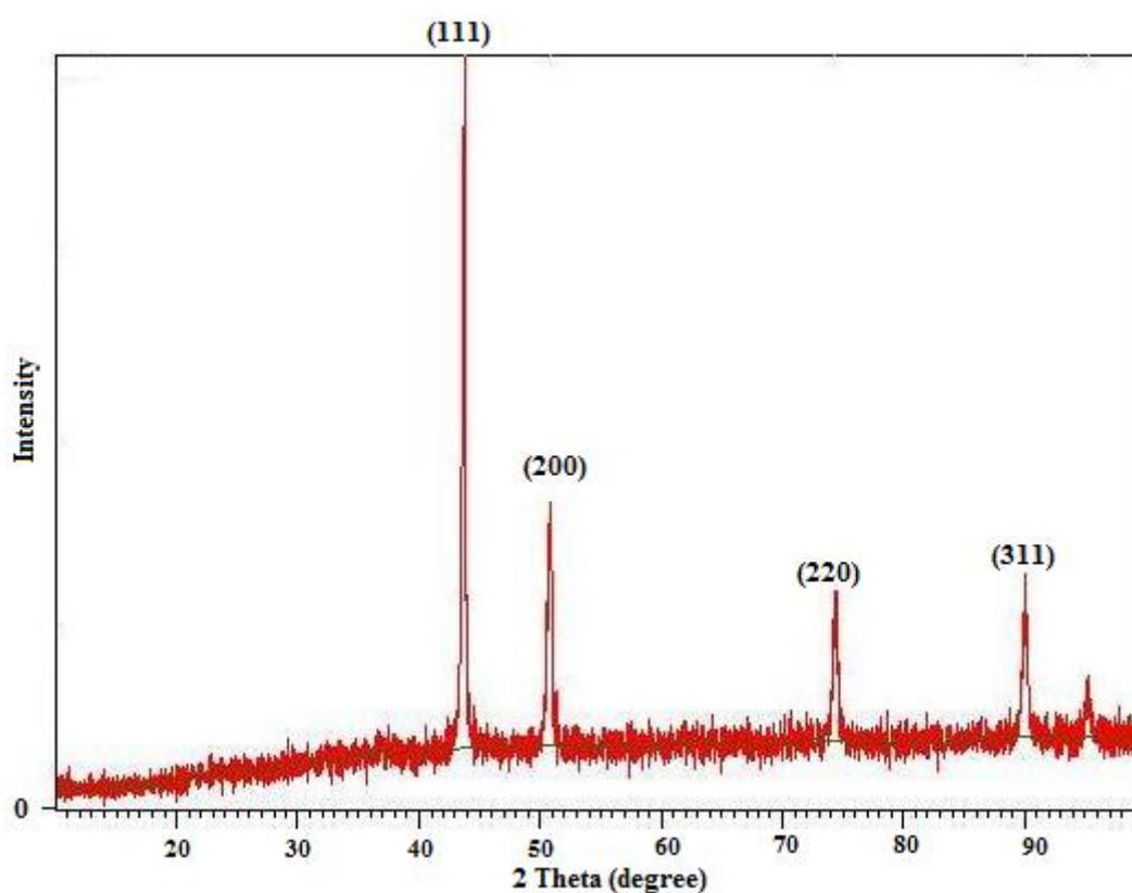
Figure 2: X-ray diffraction analysis of Copper NPs
