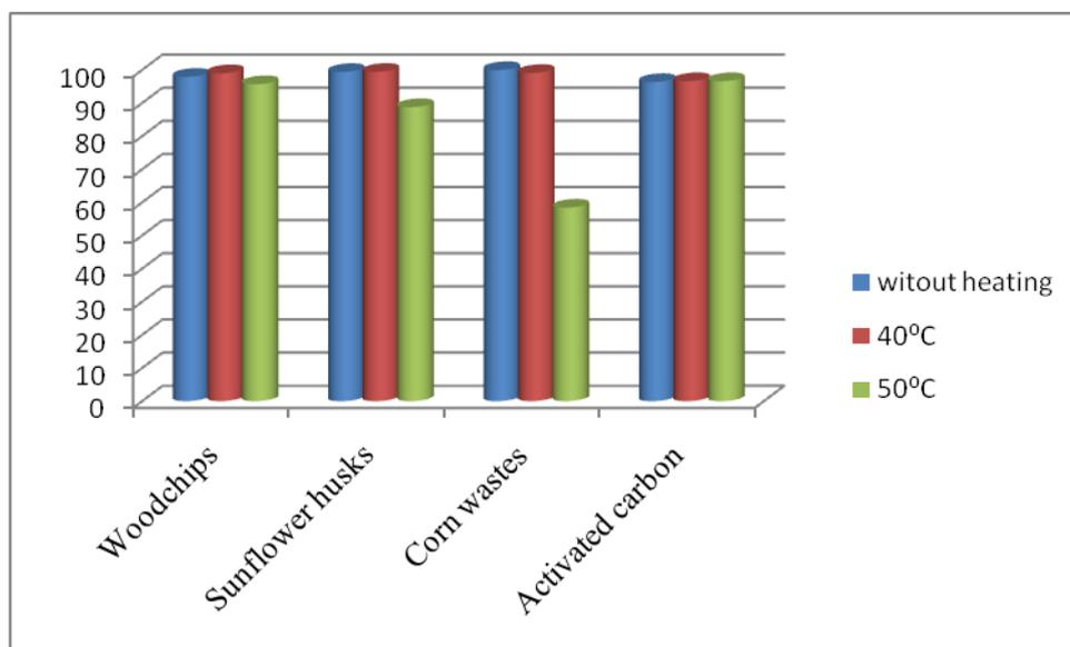
**Figure 2: Dependence of the efficiency of purification WW at adsorption temperature for 1 hour**
