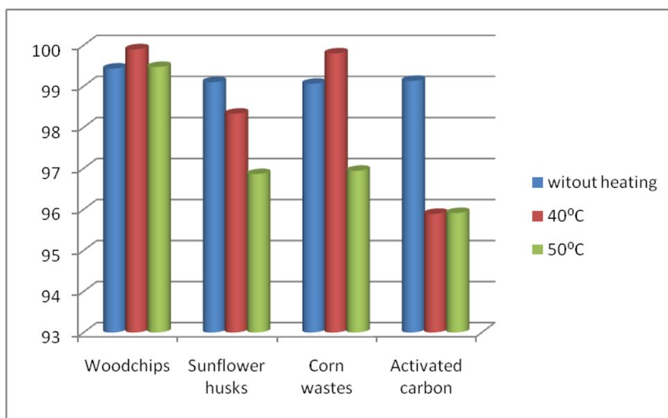
**Figure 1: Dependence of the efficiency of purification WW at adsorption temperature for 30 minutes**
