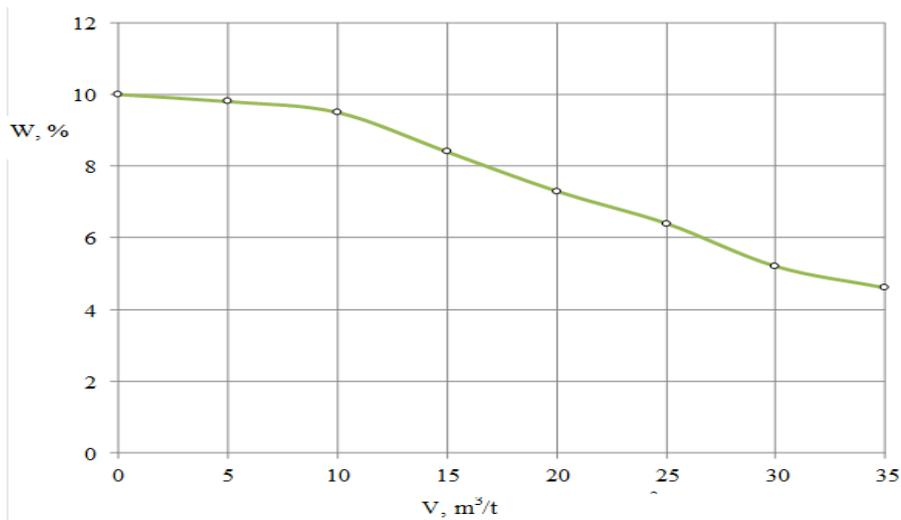
Picture 1 – Change of moisture mass fraction in the product depending on the airspeed in a solution with lactulose mass fraction of 50%
