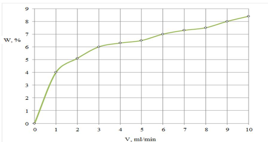
Picture 2 – Change of moisture mass fraction in the product depending on the solution feeding rate in a solution with lactulose mass fraction of 50%
