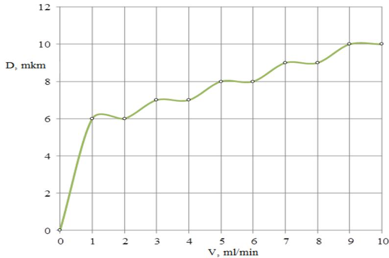
**Picture 3 – Change of dry lactulose particle size depending on the solution feeding rate at lactulose mass fraction of 50 %**
