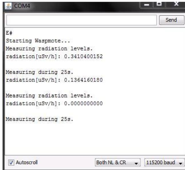
**Figure.3. Immediate recording of natural radiation**
