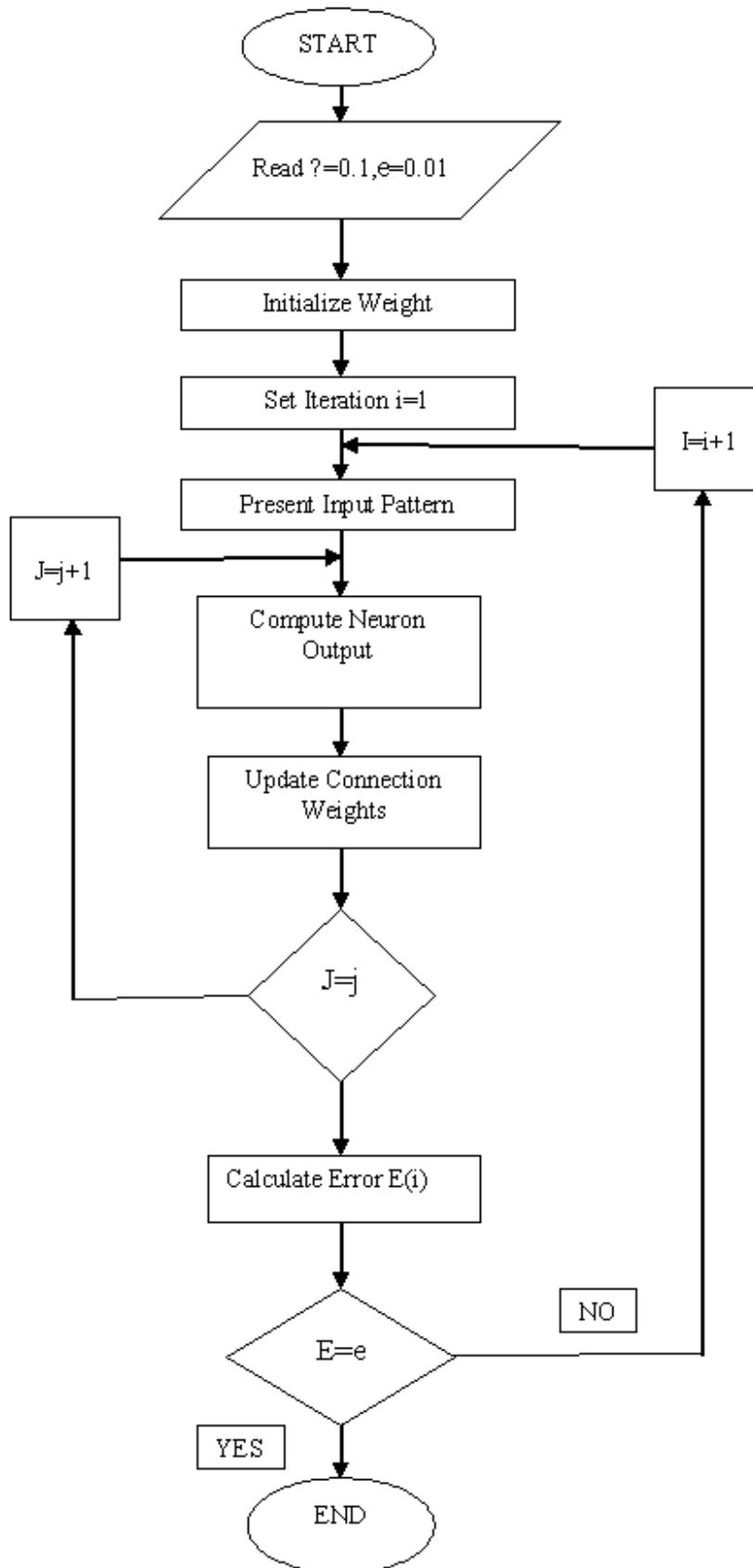
Figure 7a . Flowchart for Back Propagation Algorithm
