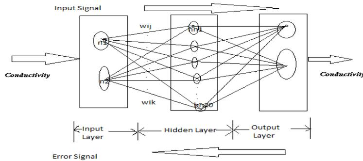
Figure 6: Multilayer Feed Forward Neural Network using Back Propagation
