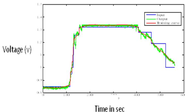
Figure 10. Tracer leak response of neural network
