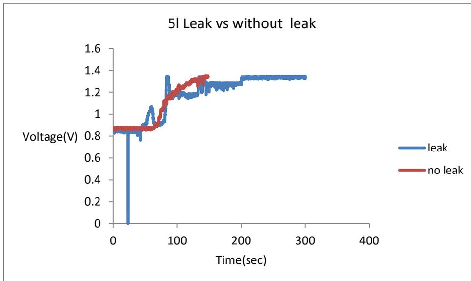
Figure 5: Response for inlet leak at 5 lpm flow rate
