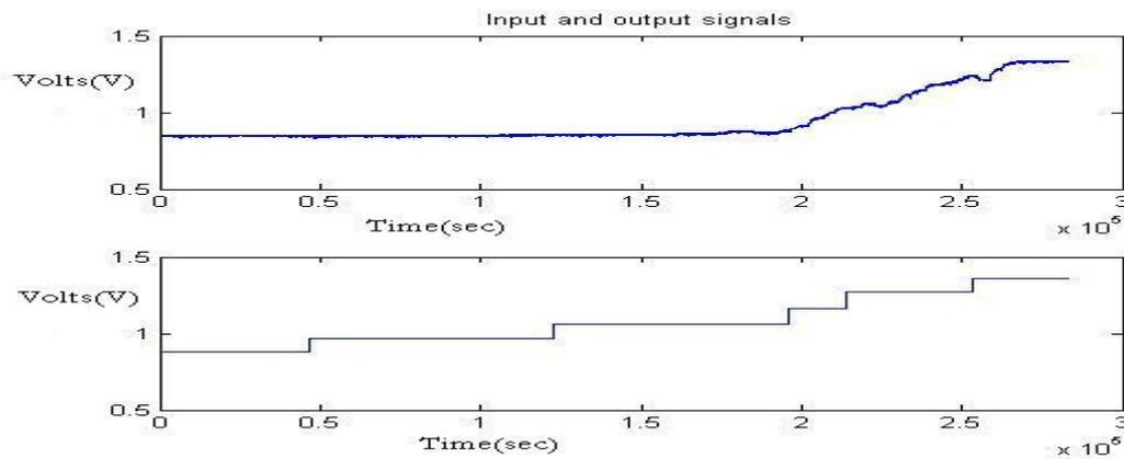
Figure 2: Open loop response for 3 lit/min water flow rate.
