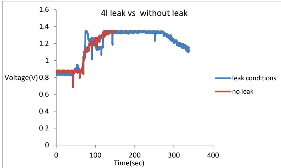
Figure 4: Response for inlet leak at 4 lpm flow rate
