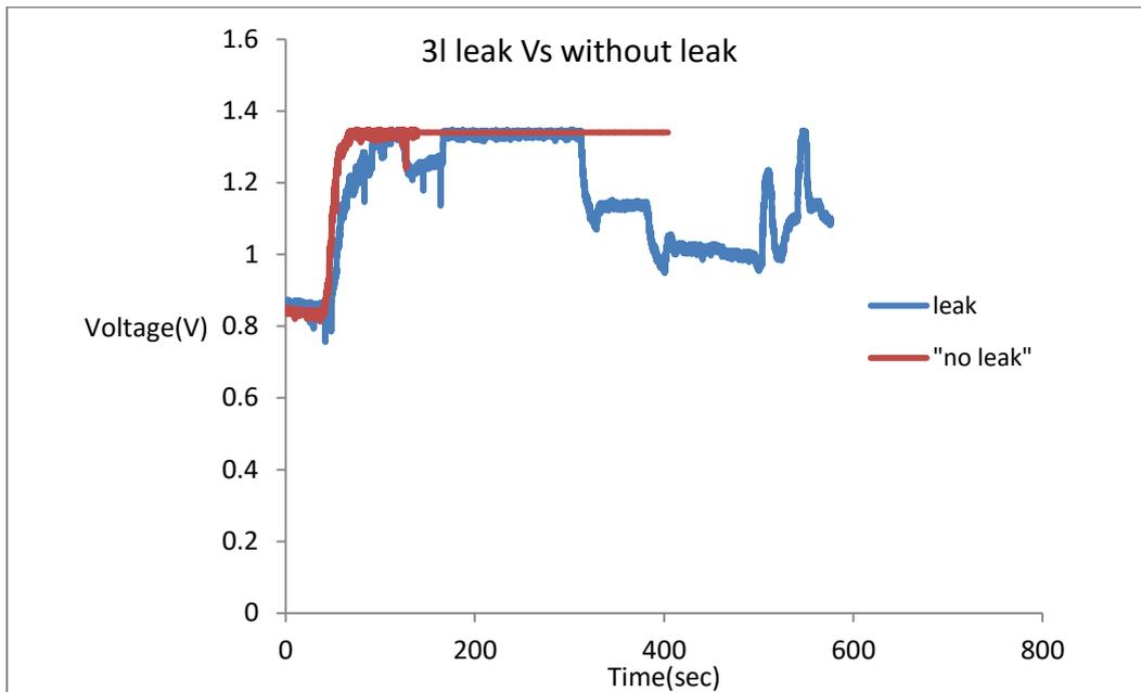
Figure 3: Response for inlet leak at 3lpm flow rate
