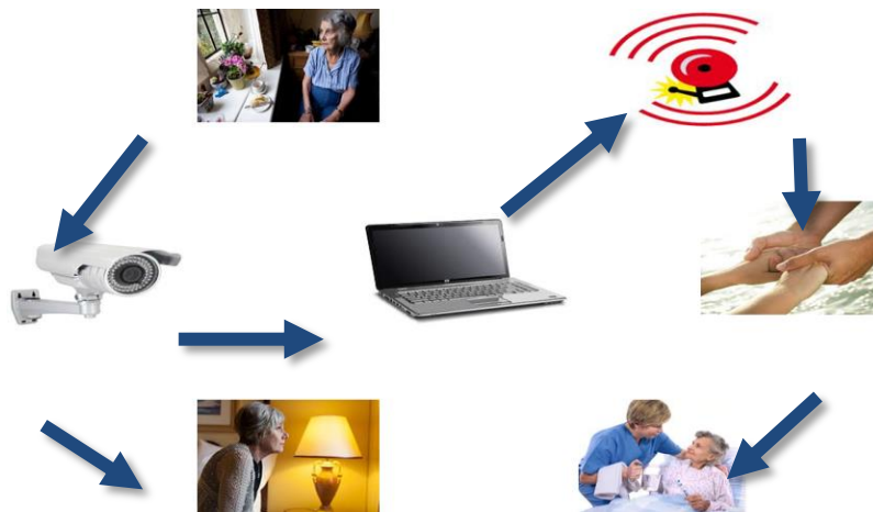
Figure 1: Typical Fall detection System
