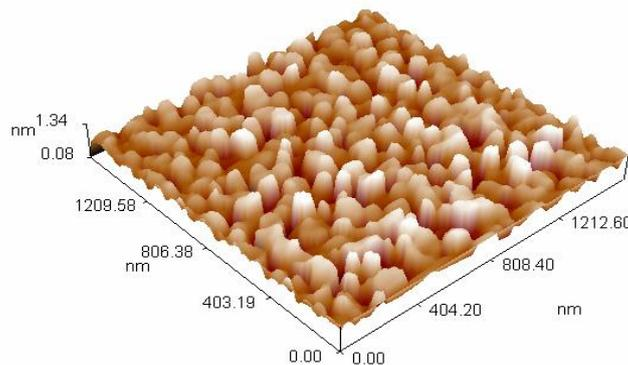
Figure (10): AFM of SD/PANI composite.
