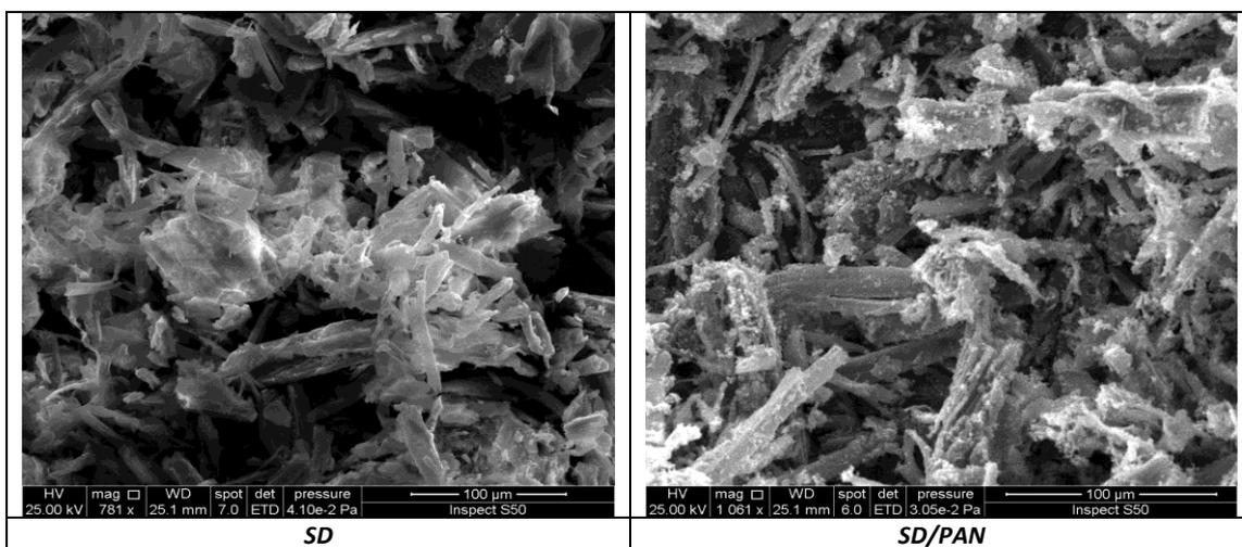
Figure (6): SEM image of the adsorbents before and after the modification.
