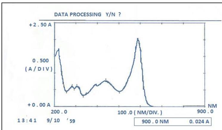
Figure (5): The  $\lambda_{max}$  of BTB dye.
