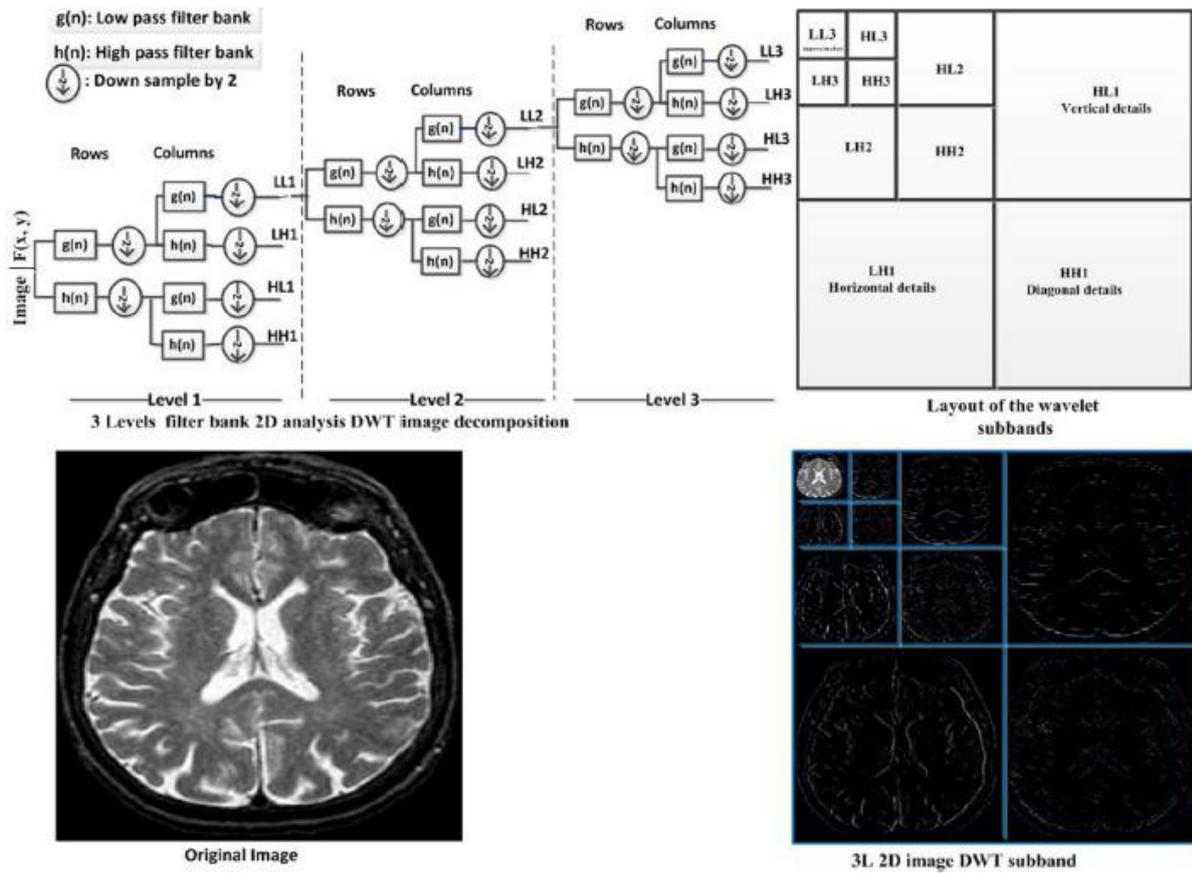
Figure 16 : Process of Discrete Wavelet Transform
