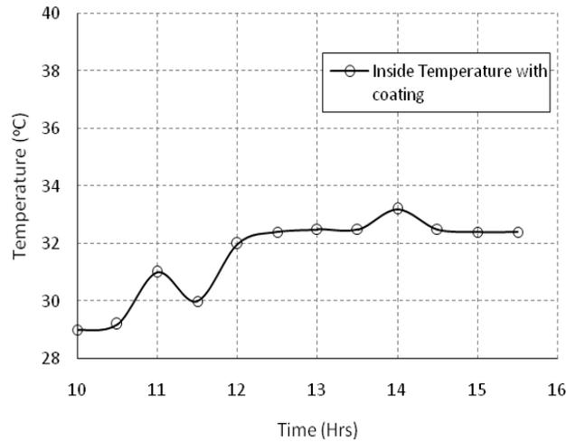
**Fig. 5. Inside temperature with coating of reflective paint on the exterior surface**
