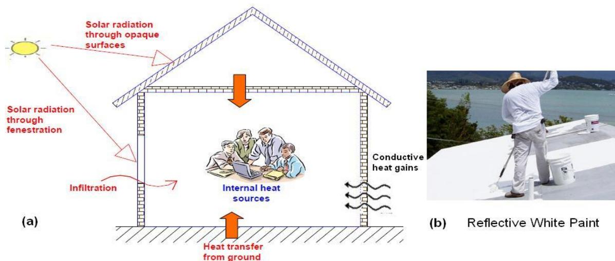
**Fig. 1 (a) Different sources for heat gain within a building (b) Applying reflective white paint on the roof surface**
