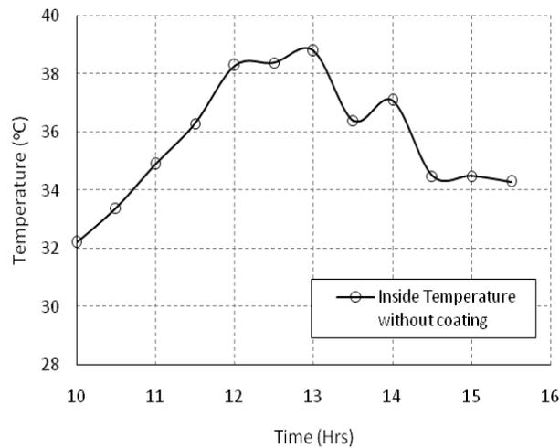
**Fig. 4. Inside temperature without coating of reflective paint on the exterior surface**
