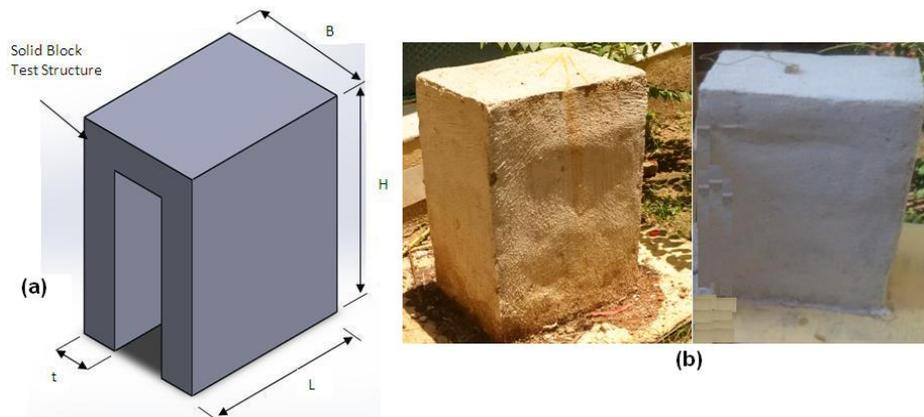
**Fig. 2. (a) Schematic model of the test structure (b) Experimental setup of the test structure with reflective paint coating**
