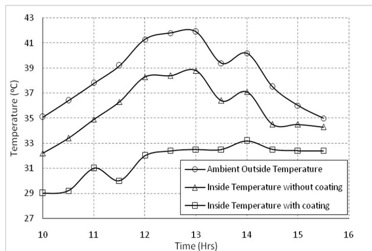
**Fig. 6. Comparison of ambient temperature, inside temperature with and without coating**
