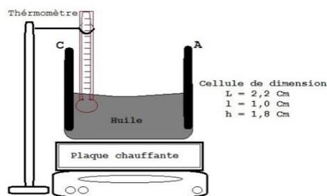
b. cell measuring the resistivity.
