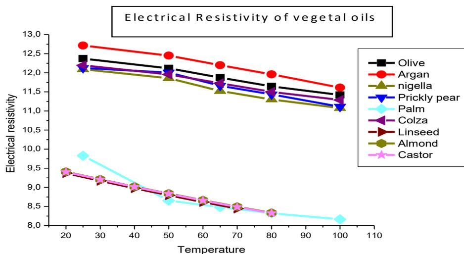
**Figure 1 : Electrical resistivity of vegetable oils (olive, argan, nigella, Prickly pear, palm, colza, linseed, almond, castor)**
