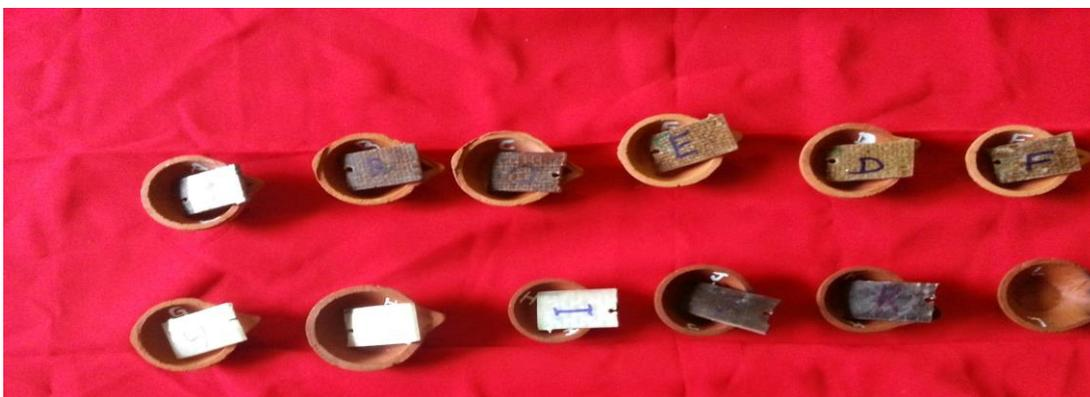
Fig c. Moisture absorption test specimens
