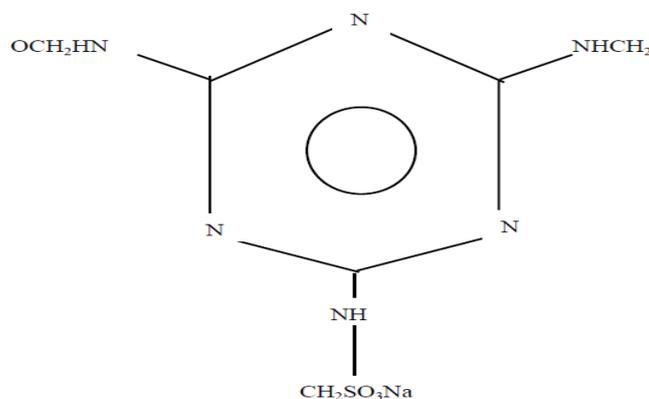
**Figure 2: Scheme of poly melamine sulfone**
