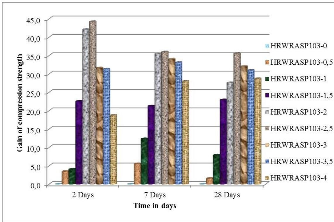
**Figure 14: Variation of gain in  $R_{mc}$  as a function of time in days**
