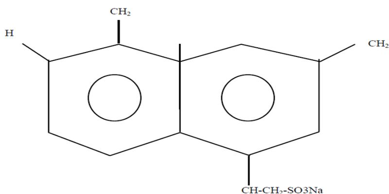
**Figure 1: Scheme of poly-naphthalene sulfone**
