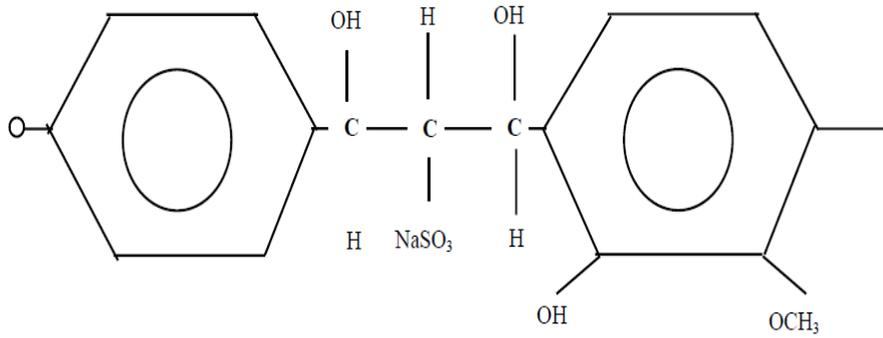
**Figure 3: Scheme of lignosulphonate of high purity**
