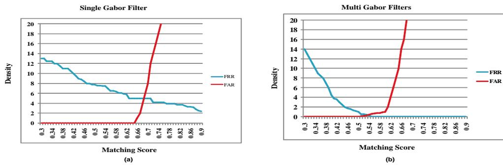
Fig 6: FAR and FRR distributions of (a) single Gabor filter; (b) multi Gabor filter
