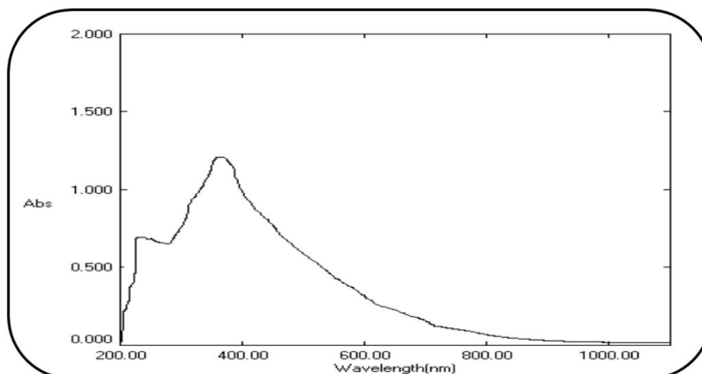
Fig (1): UV-Vis Spectrum of Ligand ( $L_1$ )
