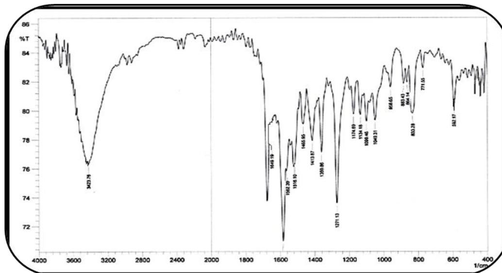
Fig(11): FT-IR of Complex [ Hg ( L<sub>2</sub> ) ]
