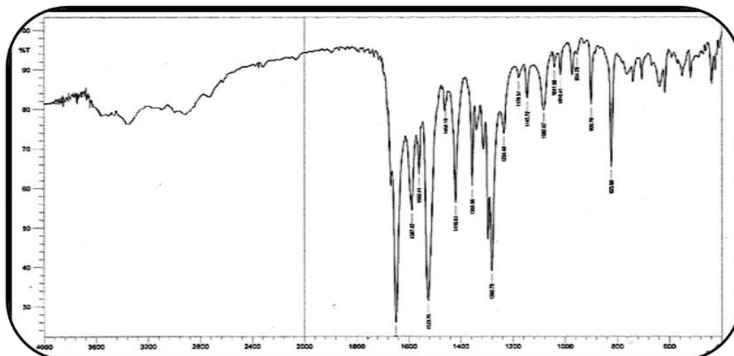
Fig(9): FT-IR of Complex [ Hg ( L<sub>1</sub> ) ]
