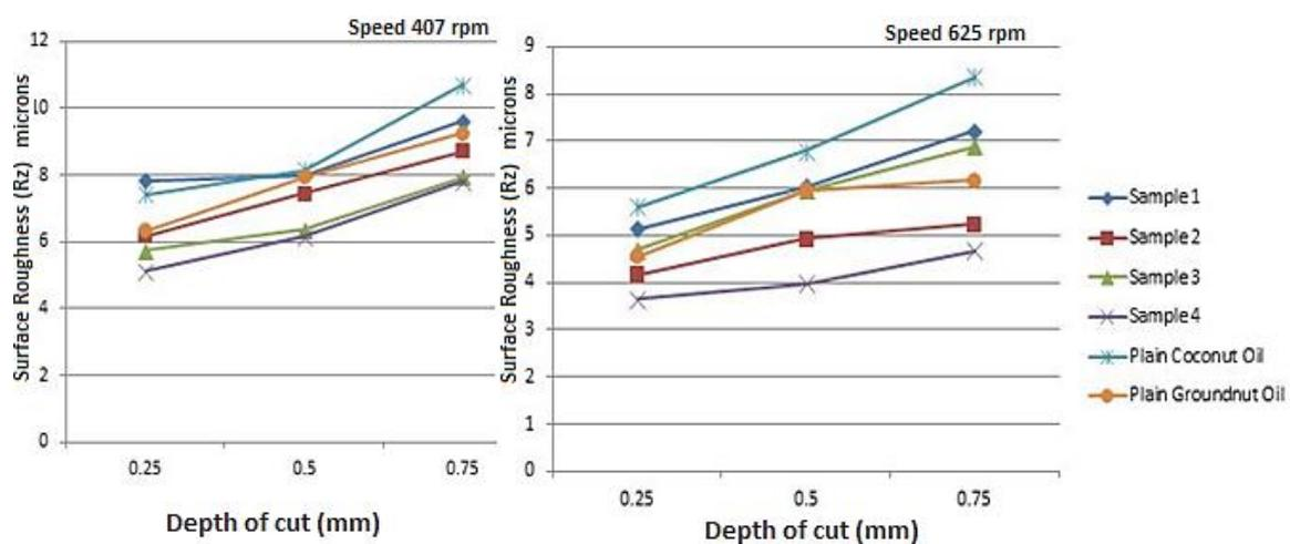
**Figure 4: Surface roughness analysis of machined surface, plotted for set parameters on lathe**
