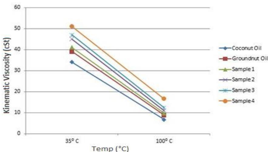
**Figure 1: Graph depicting Kinematic viscosity of lubricants at 35°C and 100°C**
