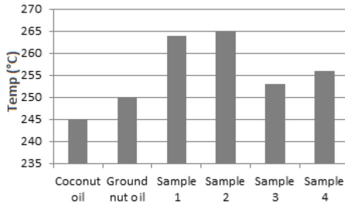
Figure 2: Flash point determination of prepared samples and base oil
