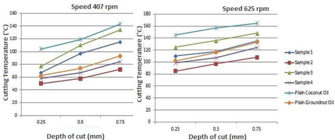
Figure 3: Cutting temperature at various depth of cuts
