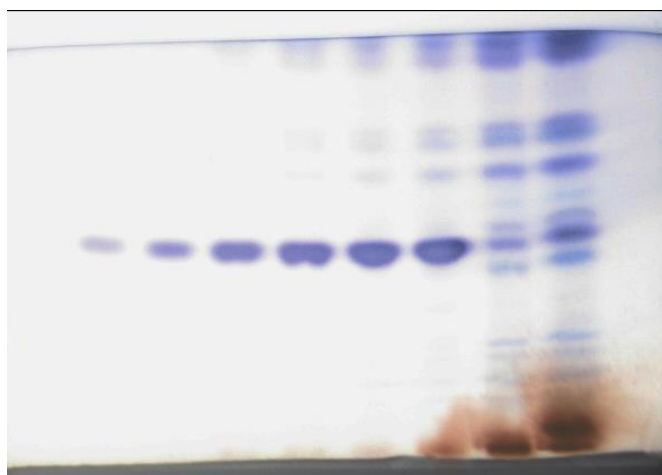
Fig 1: HPTLC chromatoplate of betulinic acid and hydroalcoholic extract of powdered bark of Madhuca longifolia after derivatization under 560 nm at different concentration 0.2, 0.4, 0.6, 0.8, 1.0 and 1.2 µg/spot standard Betulinic acid and Hydroalcoholic extract of bark of M. longifolia .
