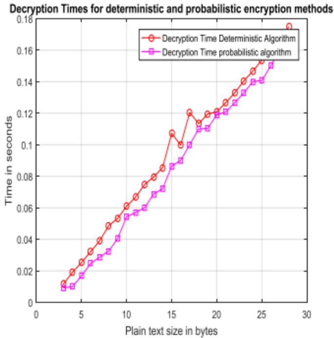
Figure 9: Deterministic Asymmetric key algorithm (RSA) vs Probabilistic Public key algorithm - decryption speed
