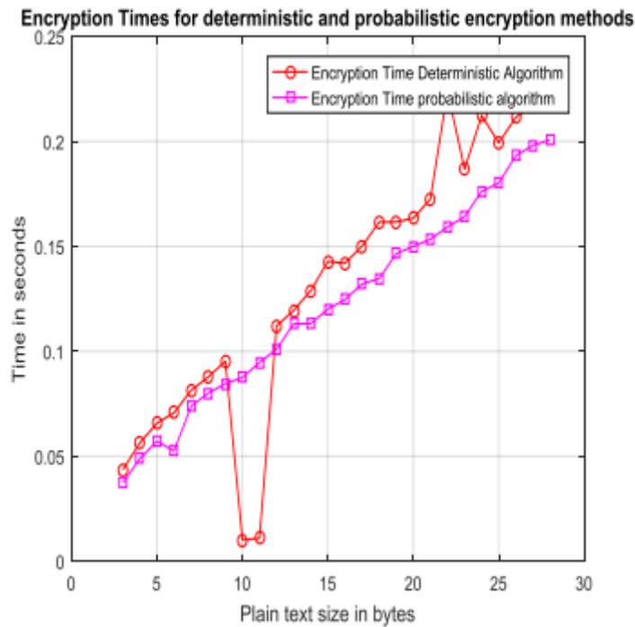
Figure 10: Deterministic Asymmetric key algorithm (RSA) vs Probabilistic Public key algorithm - encryption speed
