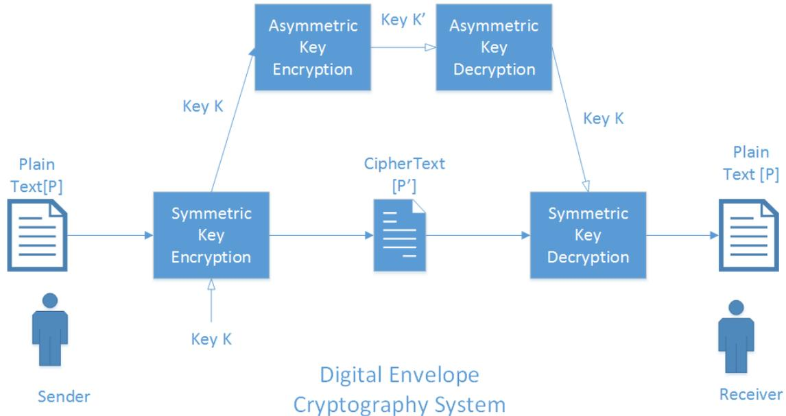
**Figure 2: Digital Envelope Cryptography System**
