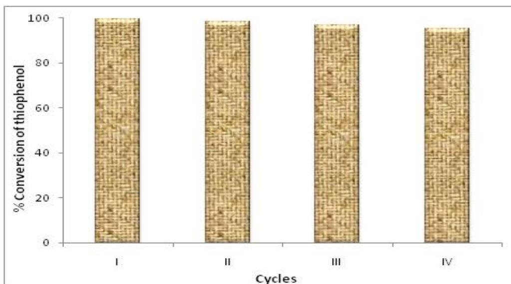
Reaction condition: thiophenol/oxidant- 2/6mmol, ACN-10ml, Catalyst-0.3g, Temp.-80°C
