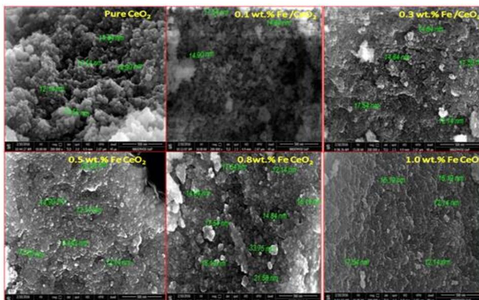
**Fig 4: FESEM images of prepared mixed oxide catalysts**
