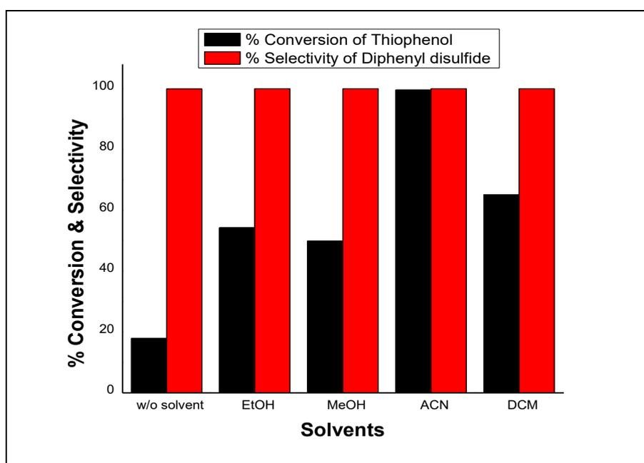
Reaction condition: thiophenol/oxidant- 2/6mmol, Solvent-10ml, Catalyst-0.3g. Temp.-80°C
