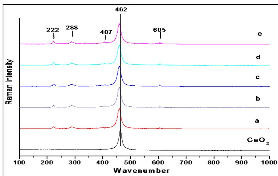
**Fig 3: Raman spectra of pure  $\text{CeO}_2$ , a) 0.1, b) 0.3, c) 0.5, d) 0.8, and e) 1.0 wt. % of  $\text{Fe}/\text{CeO}_2$  mixed oxide catalysts**
