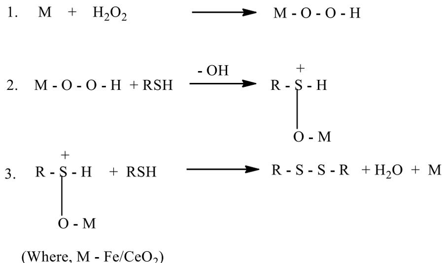
**Fig 10: Mechanism of oxidative coupling of thiophenol**
