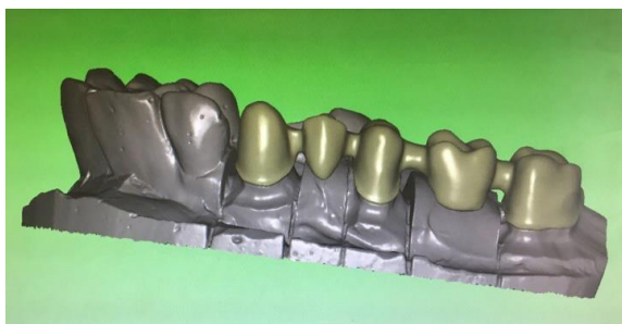
Fig 9: Modeling the frame and preparing model for the CadCam router
