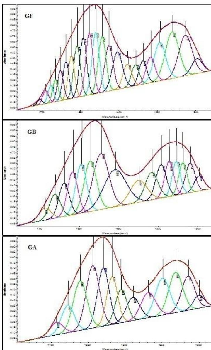
Figure 4: The component bands of amide I and amide II curve fitting of the gelatin types under investigation [based on their derivative]. The red line represent the original spectrum and the blue line represent the fitted one.
