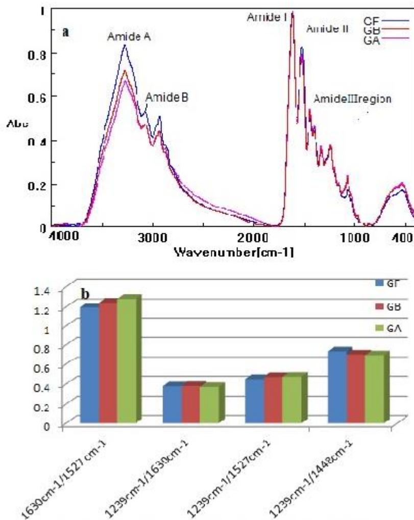
**Figure 1: ATR-FTIR spectra of gelatin types used (a) and their absorbance ratios of the bands at  $1630\text{cm}^{-1}/1527\text{cm}^{-1}$ ,  $1239\text{cm}^{-1}/1630\text{cm}^{-1}$ ,  $1239\text{cm}^{-1}/1527\text{cm}^{-1}$  and  $1239\text{cm}^{-1}/1448\text{cm}^{-1}$  (b).**
