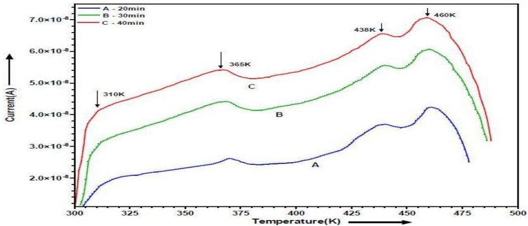
Figure 4: Thermally Stimulated Current (TSC) spectra of PAAm-PAA (1:2) blend
