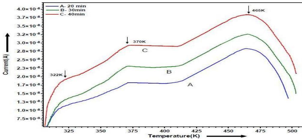
Figure 5: Thermally Stimulated Current (TSC) spectra of PAAm-PAA (2:1) blend.
