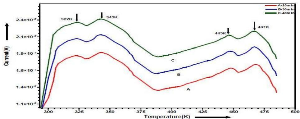
Figure 1: Thermally Stimulated Current (TSC) spectra of PAAm-PAA (1:1) blend
