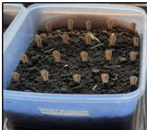
Figure 1b: Biodegradation test of bioplastics by Soil burial method in Agriculture Soil.
