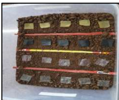
Figure 1a: Biodegradation test of bioplastics by Soil burial method in Garden S
