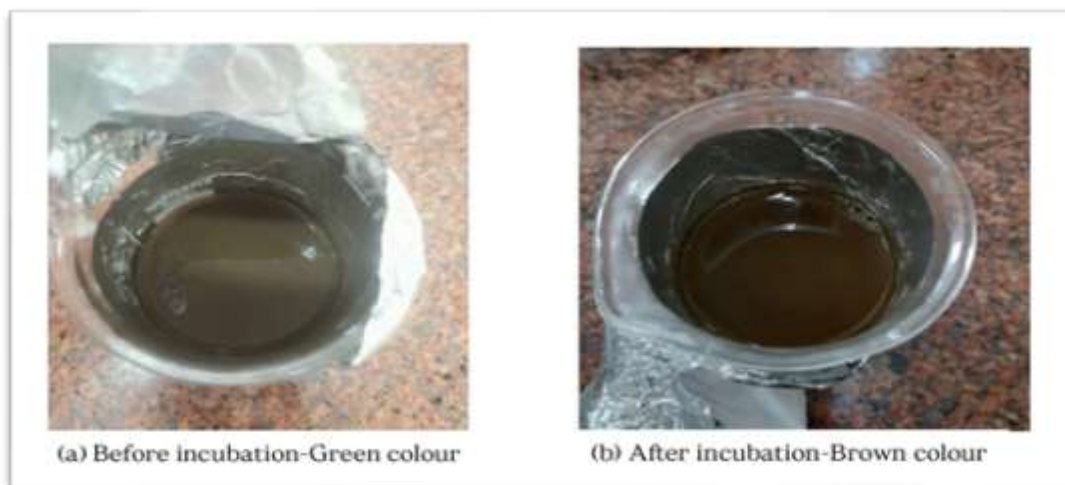
Figure 2: Color change observed during AgNP synthesis at different time intervals: (a) green before incubation, (b) brown after 24 hours of incubation.
