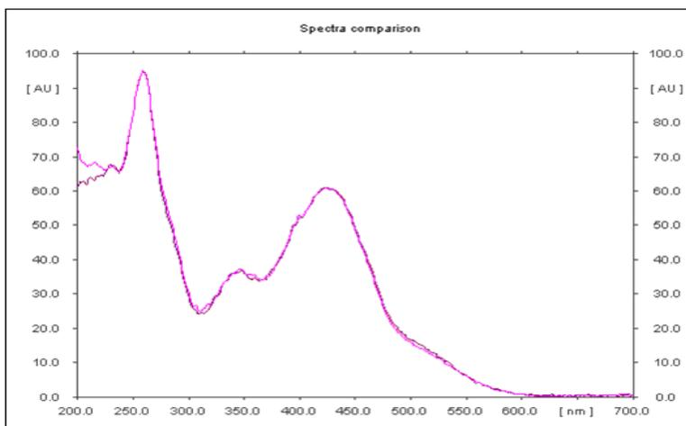
Figure No.3: Spectrum of diacerein standard and sample measured from 200 to 700 nm.
