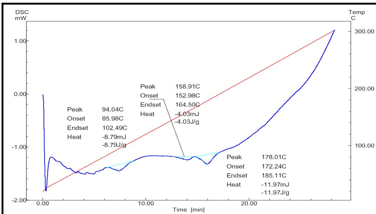
Fig. 9: Differential scanning calorimetric study of F4.
