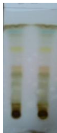
TLC of Ethanolic Extract of Ichnocarpus frutescens R.Br. on spraying with 5% H 2 SO 4
