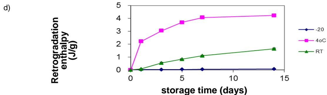
Figure 1: Retrogradation enthalpy of RD6 rice starch gels containing 30-60% water content stored at various temperatures, gel containing water 30% (a), 40% (b), 50% (c) and 60% (d), respectively.
