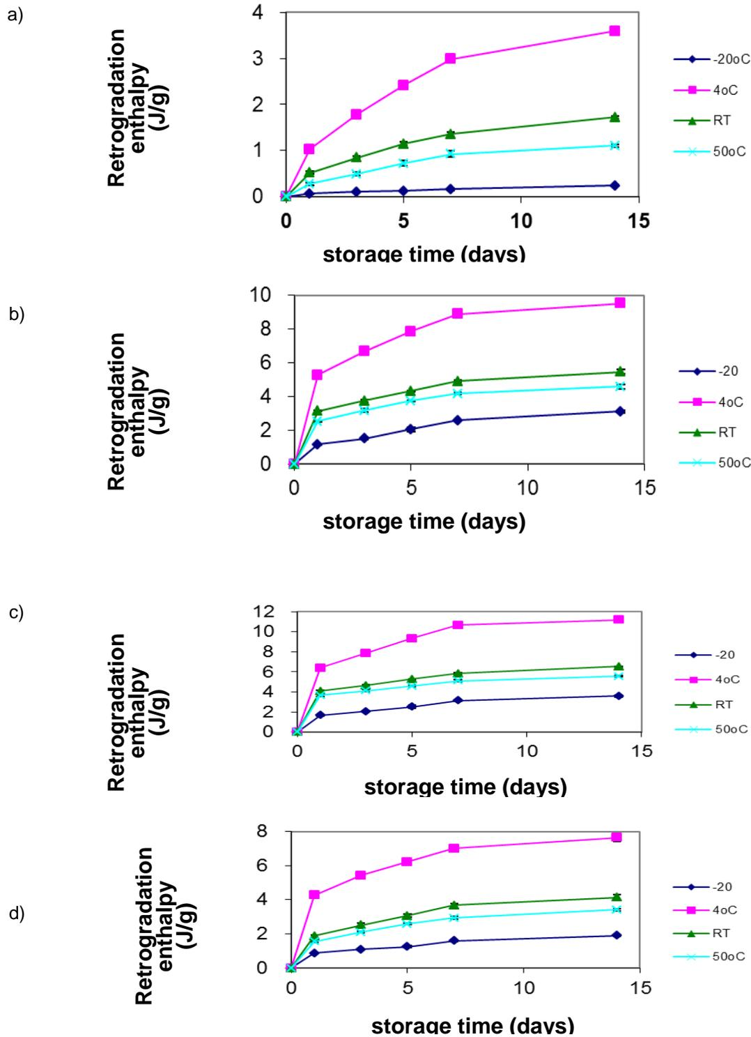
Figure 2: Retrogradation enthalpy of RD6 rice starch gels containing 30-60% water content stored at various temperature, gel containing water 30% (a), 40% (b), 50% (c) and 60% (d), respectively.
