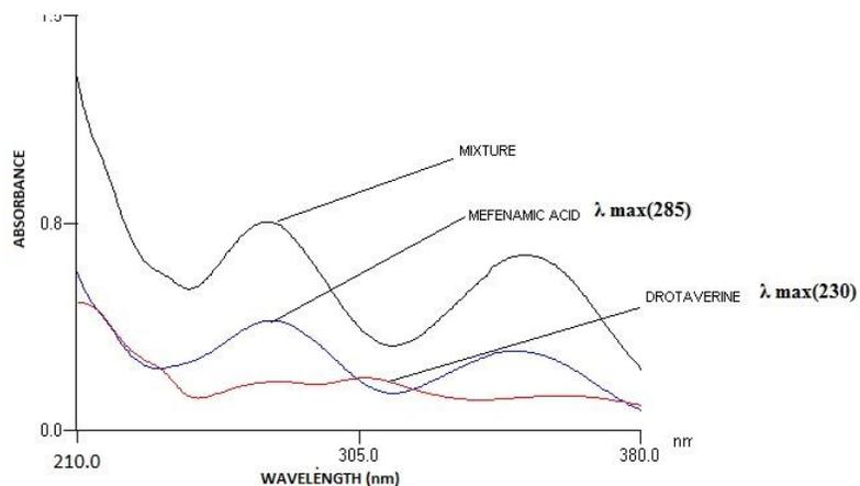
Fig.1: Overlaid UV spectra of Drotaverine Hcl, Mefenamic acid and Mixture
