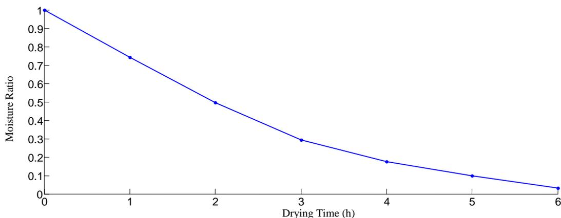
**Fig. 4: Variation of Moisture Ratio Vs Drying Time for solar drying of ginger**
