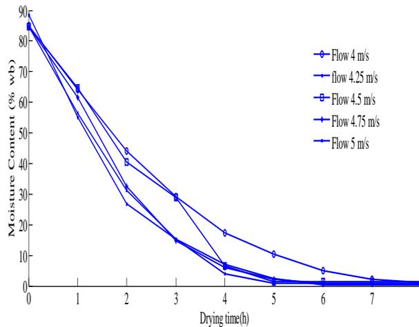
**Fig. 2: Variation of Moisture Content (%wb) Vs Drying Time for different velocity air flow rates**
