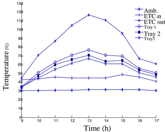
**Fig. 1: Variation of Ambient temperature, ETC inlet temperature, ETC outlet temperature, Tray1 (lower) temperature, Tray2 (middle) temperature, Tray3(upper) temperature with time of the day for air velocity flow rate of 4 m/s recorded on 06.12.12**
