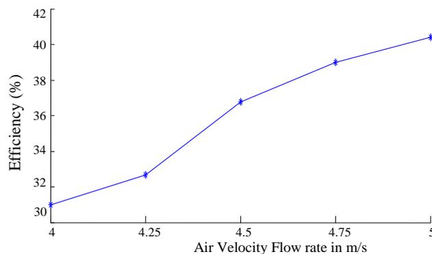
**Fig. 3: Thermal efficiency of the solar drier with evacuated tube collector at different air velocity flow rates**
