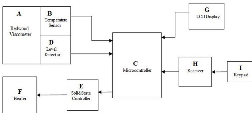
Figure (1): Block diagram of microcontroller based viscometer
