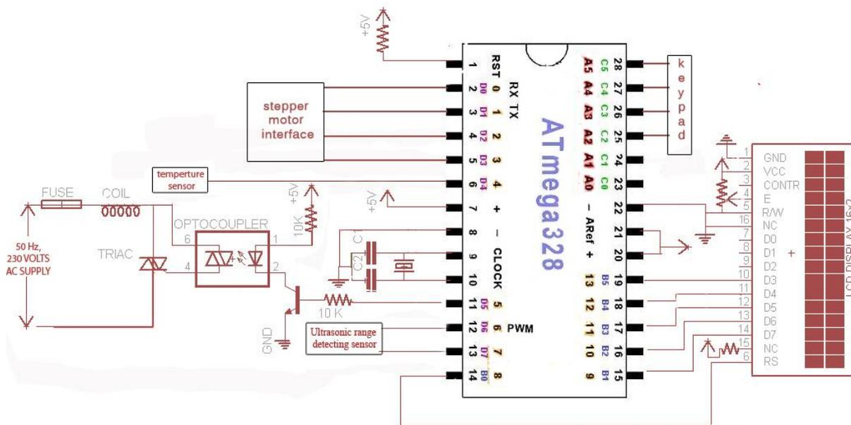
diagram for the microcontroller based viscosity measurement setup
