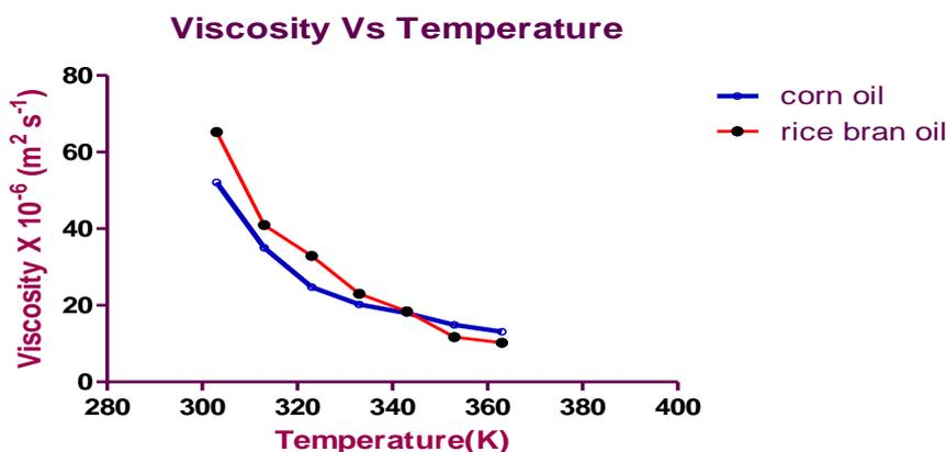
Figure (4): Variation of viscosity with temperature
