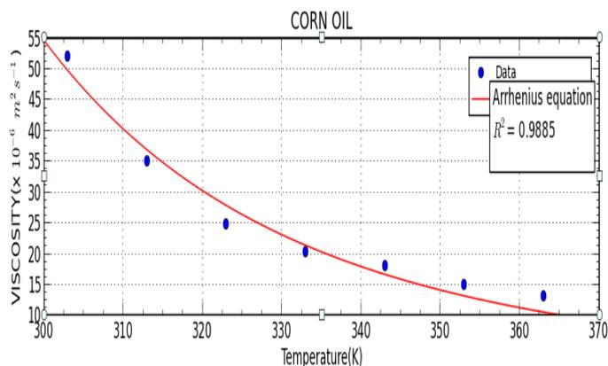
Figure (6): Regression with Arrhenius equation
