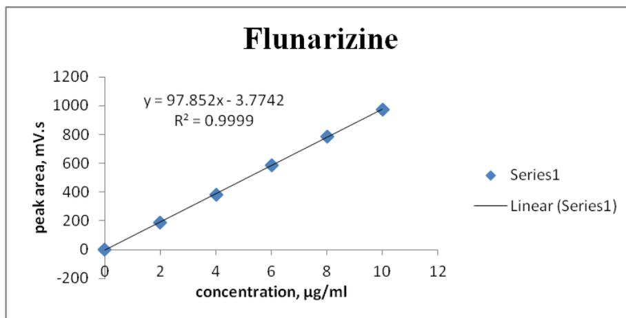
Figure.No:10 Calibration plot of Flunarizine
