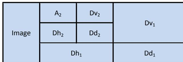
Figure 3: DWT based image decomposition
