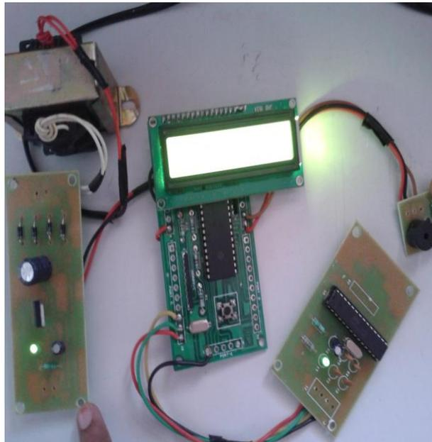
Figure 13: ZigBee Receiver
