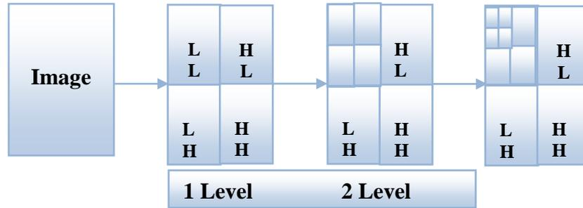
Figure 2: Discrete wavelet transforms (2D-DWT) operation
