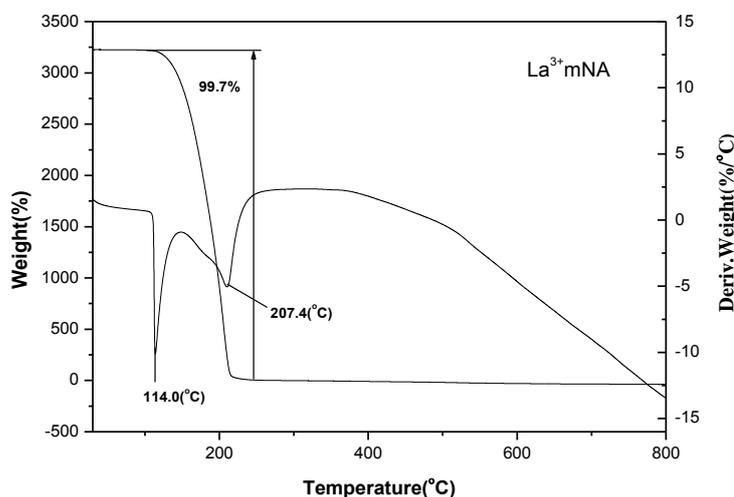
Figure 11: TG-DTA Cure of La<sup>3+</sup> doped mNA single crystal
