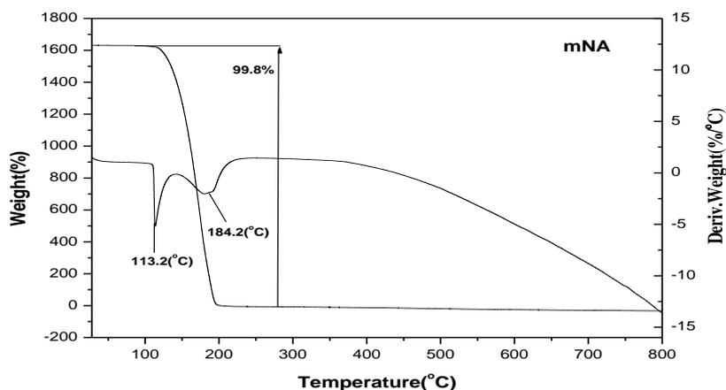
Figure 10: TG-DTA Cure of pure mNA single crystal
