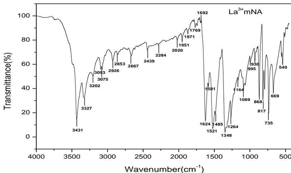
Figure 9: FT-IR Spectrum of La<sup>3+</sup> doped mNA single crystal
