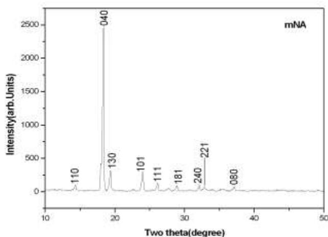
Figure 3: XRD pattern of pure mNA single crystal
