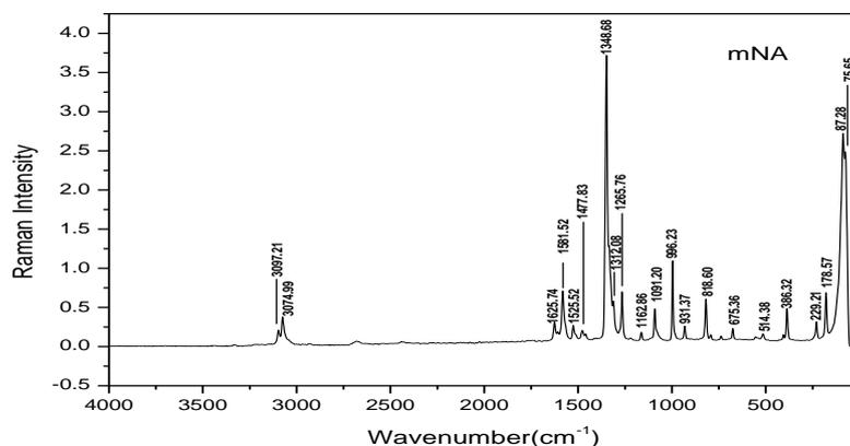
Figure 6: FT-Raman Spectrum of mNA single crystal
