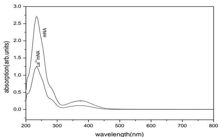
Figure 5: UV-Vis Spectrum of pure and La<sup>3+</sup> doped mNA single crystal
