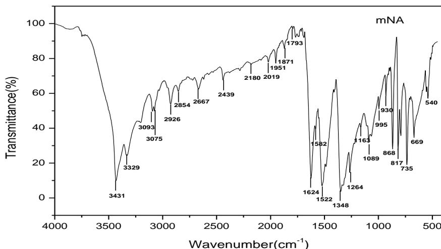
Figure 8: FT-IR Spectrum of pure mNA single crystal
