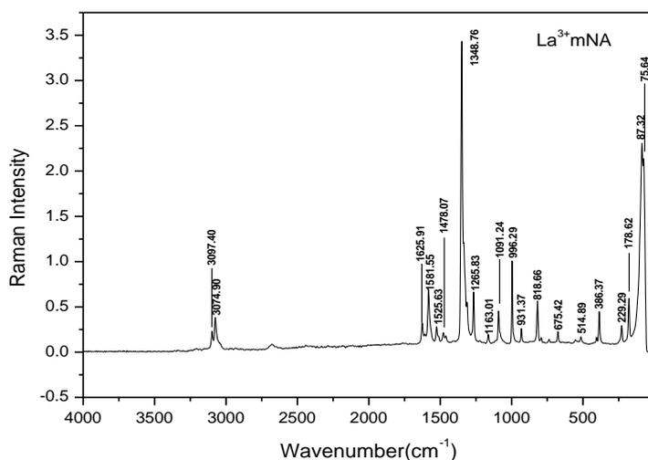
Figure 7: FT-Raman Spectrum of  $\text{La}^{3+}$  doped mNA single crystal
