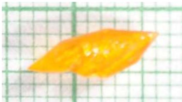
Figure 2: Photograph of La<sup>3+</sup> doped mNA crystal
