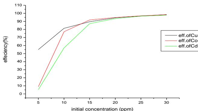
**Figure 5: effect of the initial concentration on the efficiency of removing cations**
