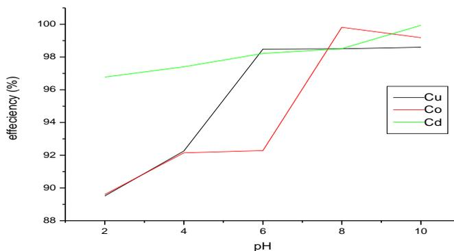
Figure 4: effect of Ph on the effeciency of removing cations
