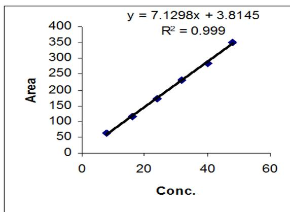
Figure 4: Linearity curve for Nebivolol hydrochloride.
