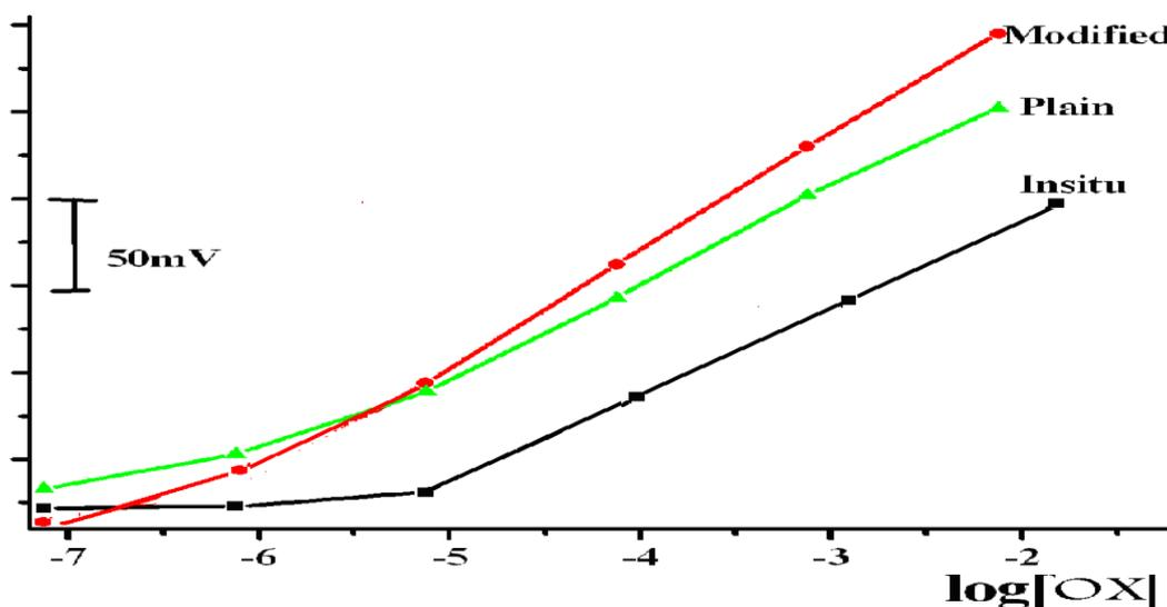
Figure 2: Potentiometric determination of OX using different PVC electrodes
