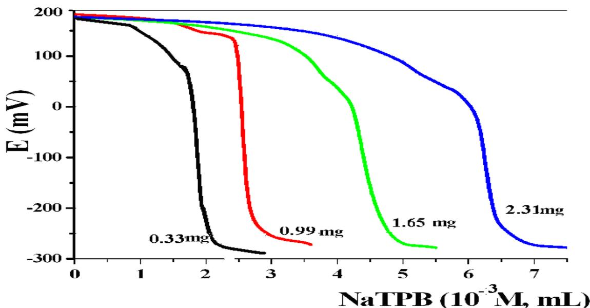
Figure 5: Potentiometric titration of OX with NaTPB using OX PVC electrode
