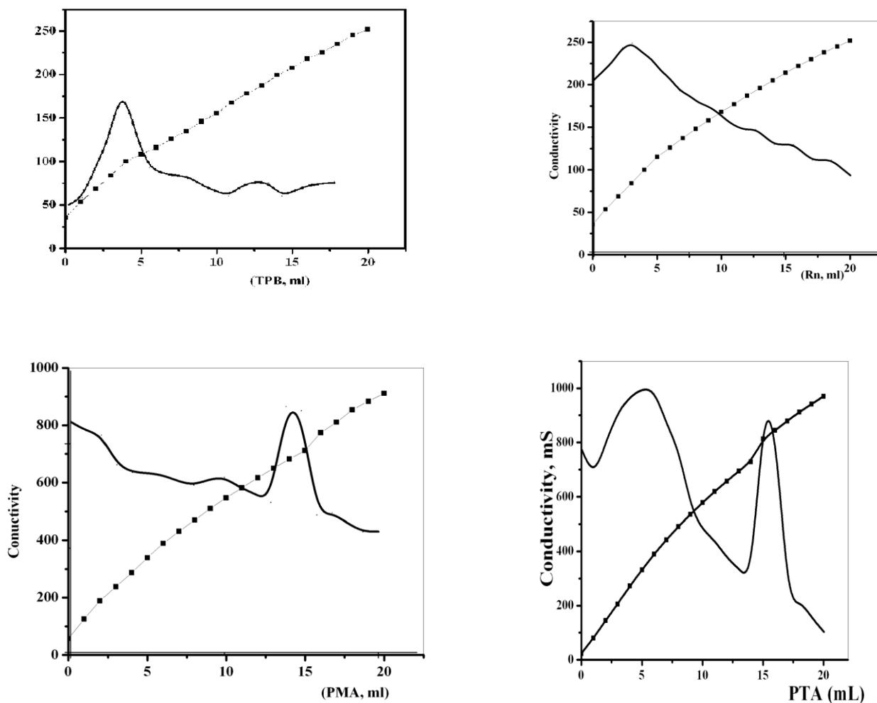
Figure 1: Conductivity measurements of different OX-ion pairs
