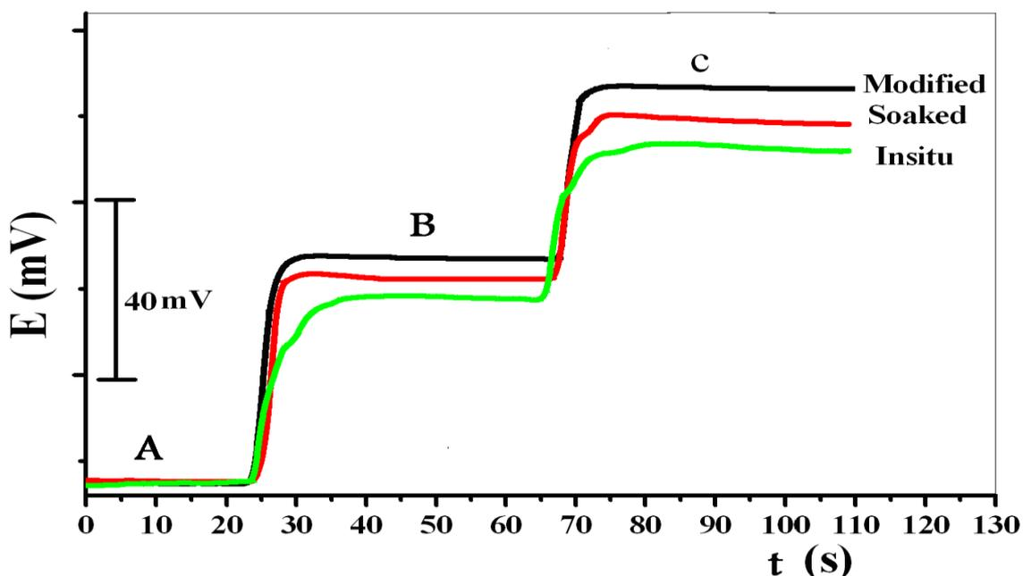
Figure 3: Dynamic response of OX PVC electrodes: (a)  $1 \times 10^{-5}$ , (b)  $1 \times 10^{-4}$  and (c)  $1 \times 10^{-3}\text{mol L}^{-1}$  OX.
