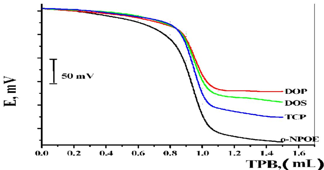
Figure 4: Effect of the electrode plasticizer on the potentiometric titration of OX with NaTPB
