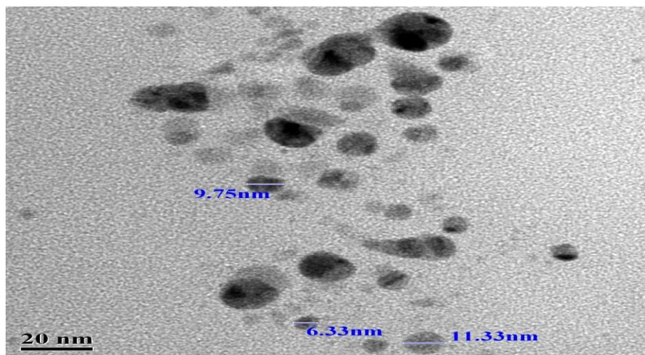
Figure 5. TEM Image of Cobalt NP showing size of nanoparticles
