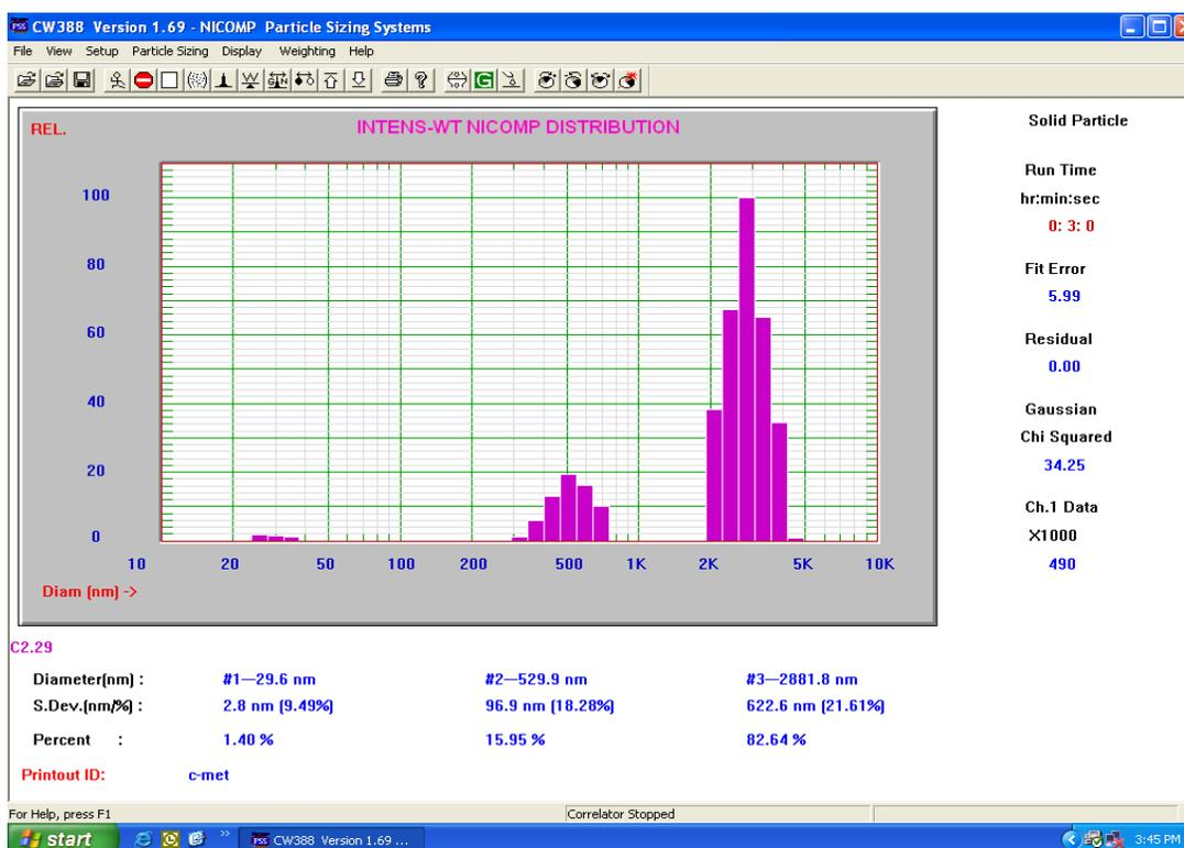
Figure 3 Particle Size Distribution Histogram of Cobalt Nanoparticles
