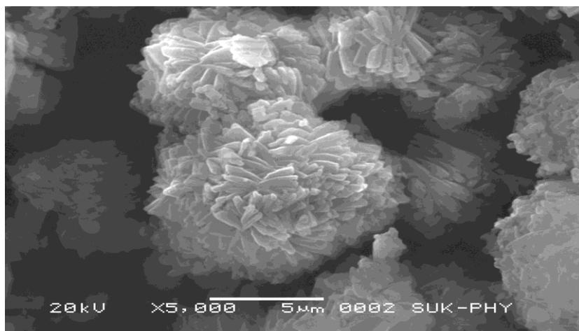
Figure 4. SEM image of Silver nanoparticles
