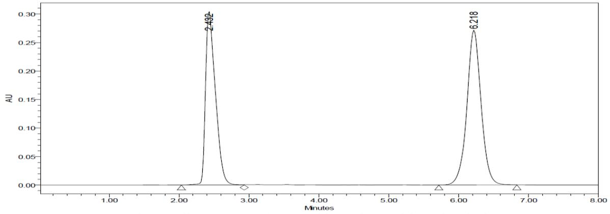
Figure-5: Chromatogram of Levocetirizine and Montelukast ( Standard)
