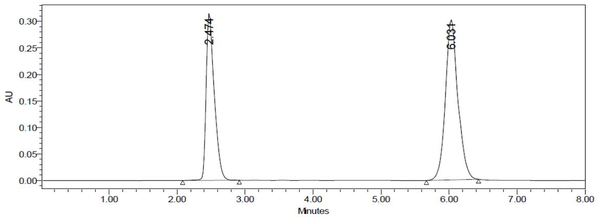
Figure 6: Chromatogram of Levocetirizine and Montelukast ( Sample)
