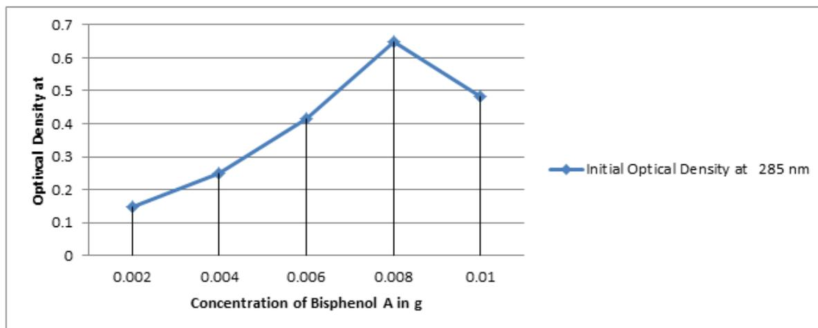
**Figure 1: Optical Density values representing the initial concentration of BPA**
