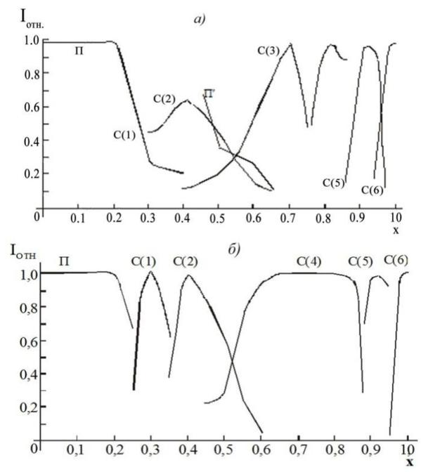
Figure 4: Phase diagrams of the systems  $(1-x)\text{NaNbO}_3-x\text{Ca}_2\text{Nb}_2\text{O}_7$  (a),  $(1-x)\text{NaNbO}_3-x\text{Sr}_2\text{Nb}_2\text{O}_7$  (b).
