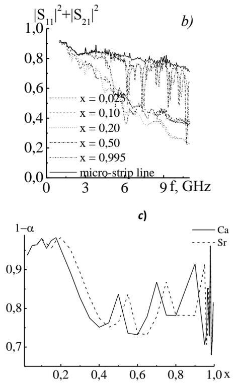
Figure 3: Relationship of losses (absorption) of microwave energy in the strip line without specimens (continuous lines) and with the specimens (dotted lines and dash-dot lines) of SS systems  $(1-x)\text{NaNbO}_3-x\text{Ca}_2\text{Nb}_2\text{O}_7$  (a),  $(1-x)\text{NaNbO}_3-x\text{Sr}_2\text{Nb}_2\text{O}_7$  (b), Relationships of losses (absorption) of microwave energy of SS of the studied systems (c).
