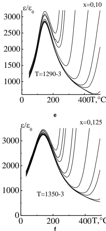
**Figure 7: Temperature relationships of dielectric permeability ( $\epsilon/\epsilon_0$ ) of the studied object for various contents of  $\text{Ca}_2\text{Nb}_2\text{O}_7$  – (a, b, c) and  $\text{Sr}_2\text{Nb}_2\text{O}_7$  – (d, e, f).**
