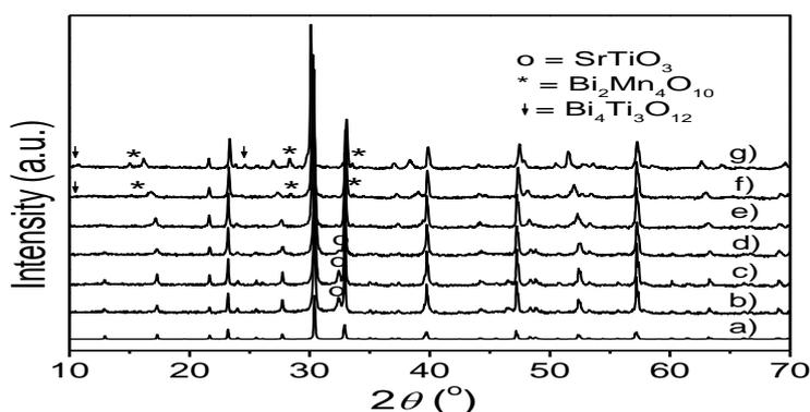
Figure 1: X-Ray Diffraction (XRD) patterns of Aurivillius phases  $\text{Sr}_{1-x}\text{Bi}_{3+x}\text{LaTi}_{4-x}\text{Mn}_x\text{O}_{15}$  were synthesized by hydrothermal technique. a)  $\text{SrBi}_4\text{Ti}_4\text{O}_{15}$  [11], b)  $x = 0$ , c)  $x = 0.2$ , d)  $x = 0.4$ , e)  $x = 0.6$ , f)  $x = 0.8$ , g)  $x = 1$ .
