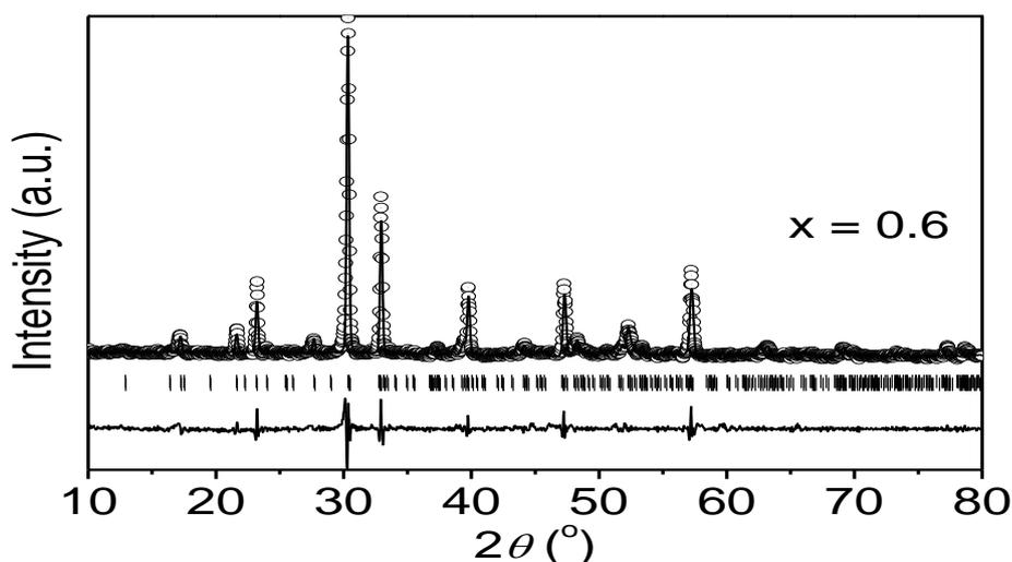
Figure 2: Le Bail plot of XRD powder of  $\text{Sr}_{1-x}\text{Bi}_{3+x}\text{LaTi}_{4-x}\text{Mn}_x\text{O}_{15}$  with  $x = 0.6$  synthesized by hydrothermal technique. Observed XRD intensity (circle), calculated data (solid line), and the difference of patterns,  $y_{\text{obs}} - y_{\text{cal}}$  (solid line on the bottom curve). The tick marks represent the positions of allowed Bragg reflections in the phase of  $A2_1am$ .
