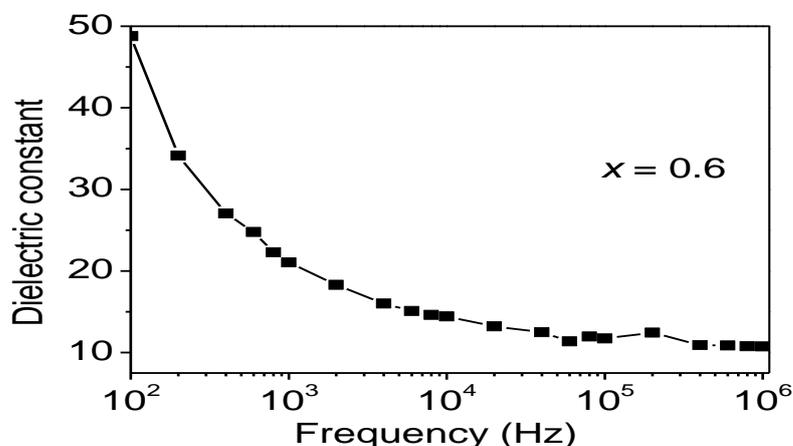
**Figure 4: Frequency dependence of dielectric constant of  $\text{Sr}_{1-x}\text{Bi}_{3+x}\text{LaTi}_{4-x}\text{Mn}_x\text{O}_{15}$  with  $x = 0.6$  synthesized by hydrothermal technique.**
