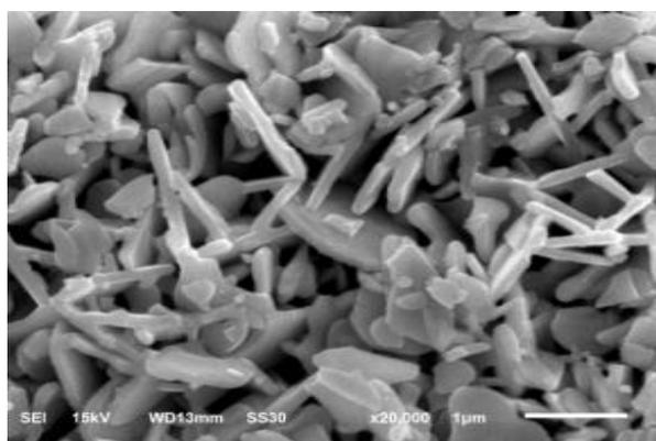
**Figure 3: SEM micrographs of  $\text{Sr}_{1-x}\text{Bi}_{3+x}\text{LaTi}_{4-x}\text{Mn}_x\text{O}_{15}$  with  $x = 0.6$  synthesized by hydrothermal technique.**
