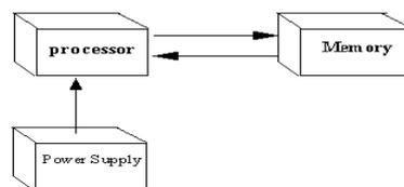
**Fig (2) Architecture of PLC**
