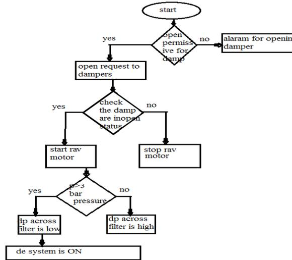
The cleaning of Filter bags carried out automatically and in a sequential manner, there are four main components involved in effective cleaning.
