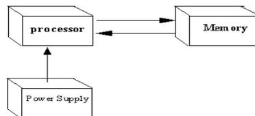
**Fig (2) Architecture of PLC**
