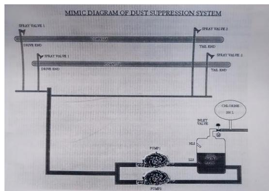
Fig (4) Block diagram of dust suppression
