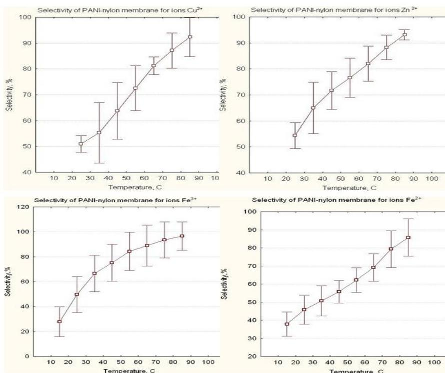
Figure 1: The dependence of selectivity of the membrane nylon-PANI from the solution temperature for metal ions:  $Fe^{3+}$ ,  $Fe^{2+}$ ,  $Cu^{2+}$ ,  $Zn^{2+}$ .
