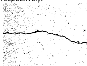
Fig.4. Conversion of gray scale to binary image
