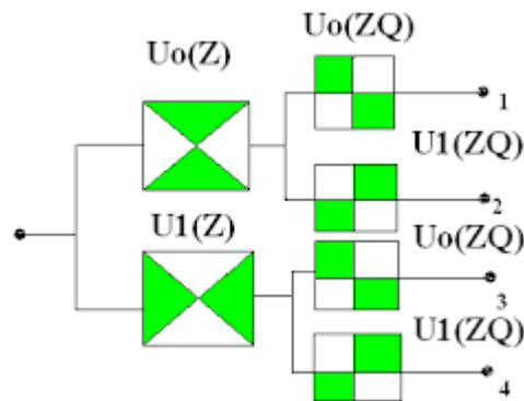
**Figure 2: Four-channel non-subsampled directional filter bank.**
