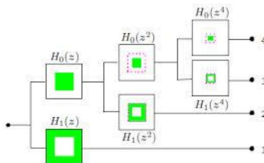
Figure 1: Three-stage non-subsampled pyramid decomposition.
