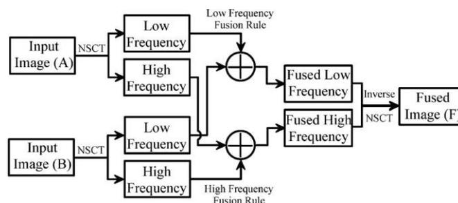
Figure 3: Block diagram of proposed multimodal medical image fusion framework.
