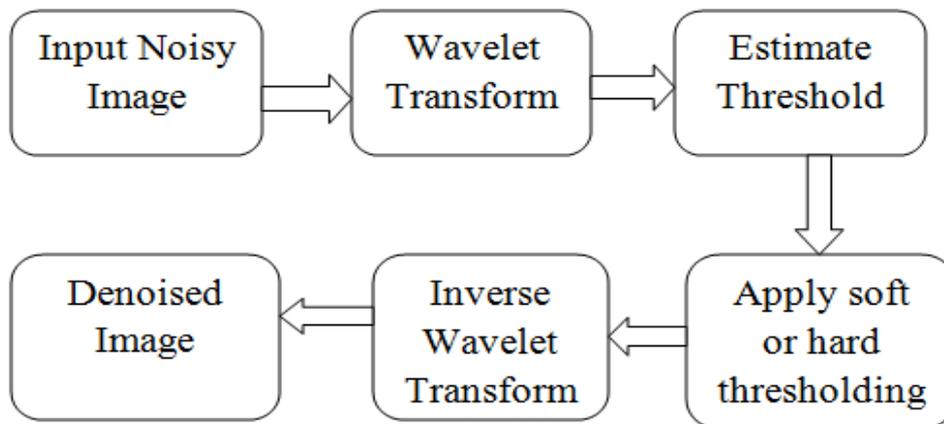
FIG.2. Block Diagram of Image Denoising Using Wavelet Transform
