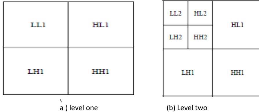
FIG.1 Image Decomposition by using DWT
