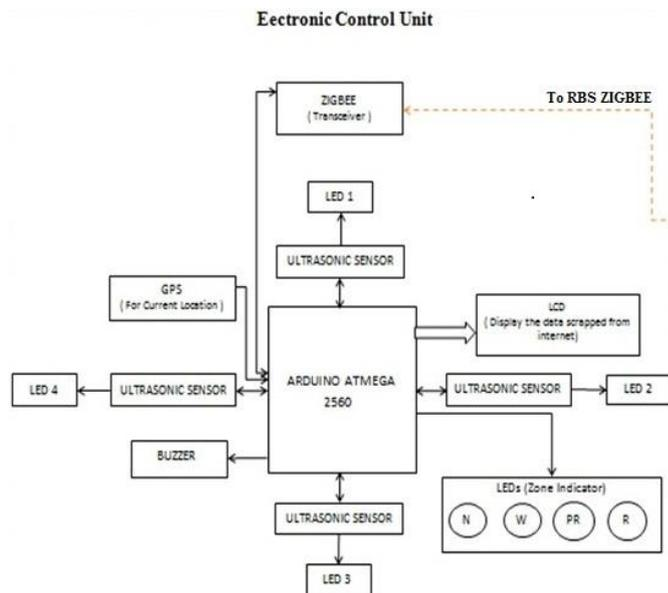
**Fig.1 Electronic control Unit(ECU)**
