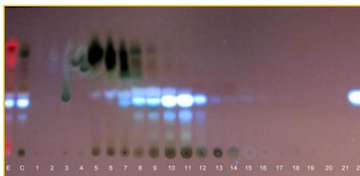
**Figure 3: TLC chromatogram of fractions after isolation with vacuum liquid chromatography. Note: stationary phase silica gel GF<sub>254</sub>, mobile phase chloroform-ethyl acetate (6:4) and visualization with UV light  $\lambda$  366 nm**
